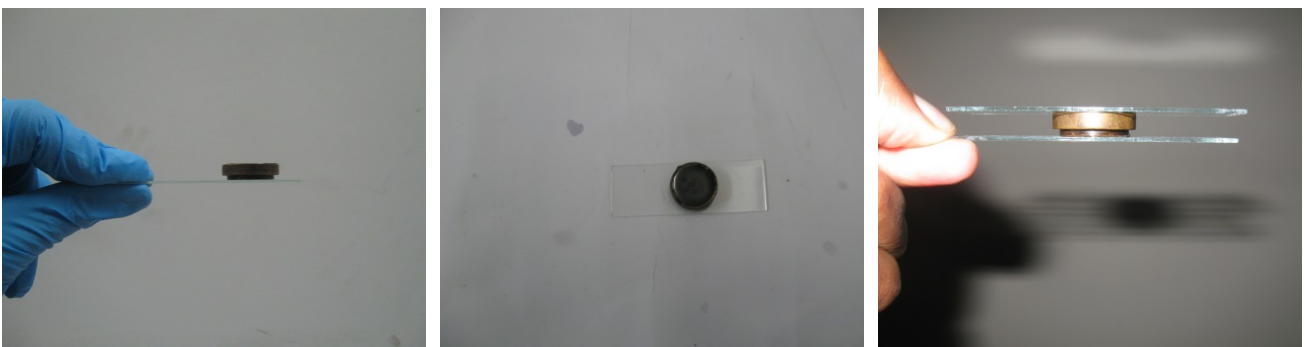
Figure 3: Bitumen inside a brass ring.
