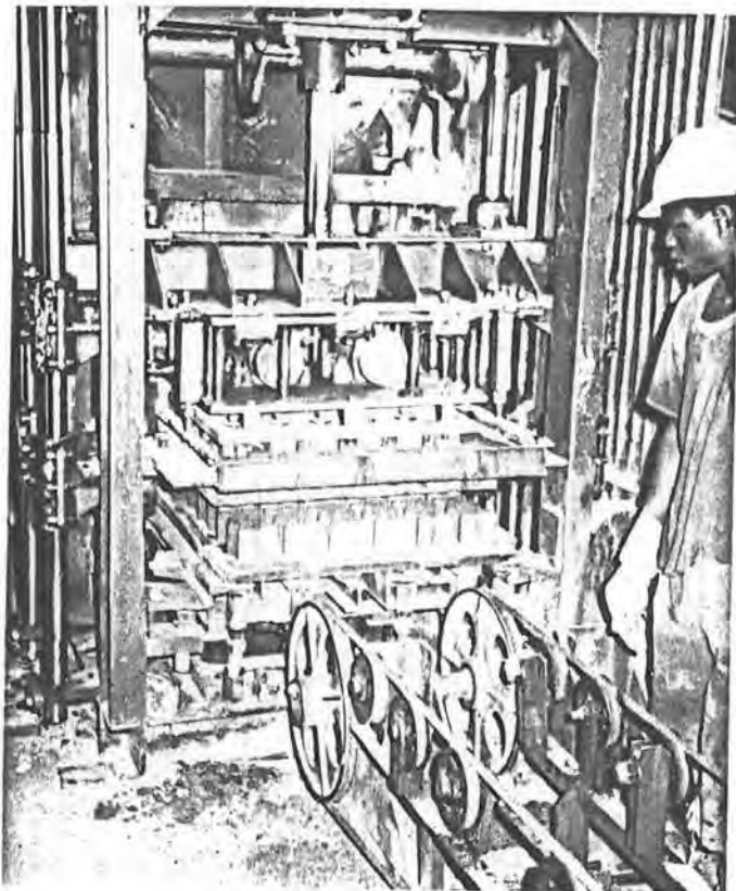
FIGURE 12.3 "LAYING HEAD" OF BLOCK MAKING MACHINE
