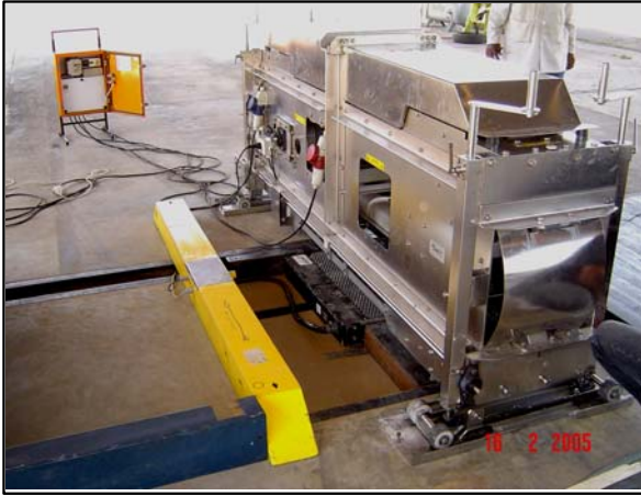
Figure 3 Model Mobile Load Simulator (MMLS3) on the SIM device at Gauteng Department of Public Transport, Roads and Works (GDPTRW) Koedoesport facility.
