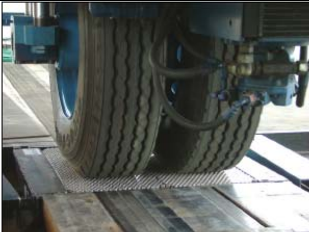
Figure 5 Heavy Vehicle Simulator (HVS) full-scale dual tyres on the rough-textured (RT) SIM surface.
