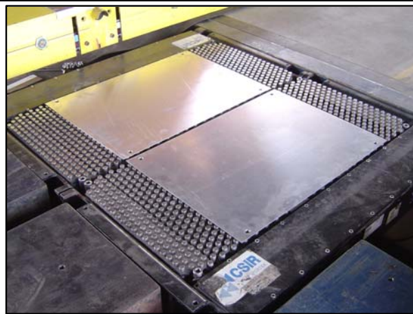
Figure 6 Artificial smooth (S) test surface showing the aluminium plate (0.9 mm) fixed on the corners of the SIM surface, before full-scale tyre testing.
