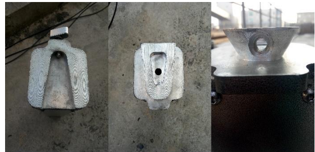
Fig.3 The mortise-tenon joints between two arms
