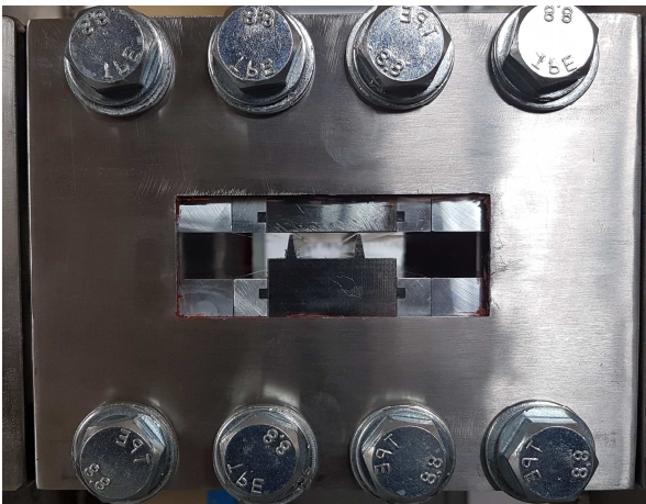
Figure 3 View of the test rig with the peephole intended for optical measurements
