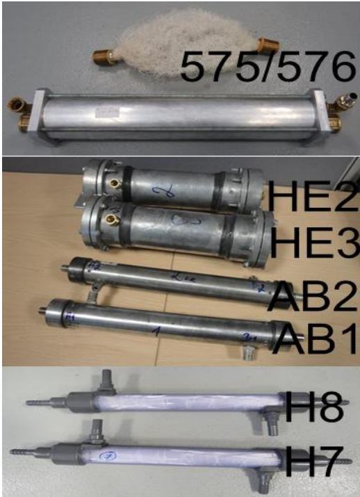
Fig.3 Polymer Hollow Fibre Heat Exchangers(PHFHE)
