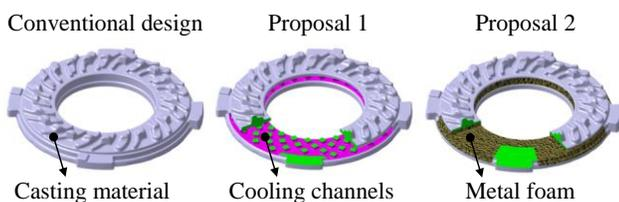
**Figure 9** Lightweight design proposals of dry clutch pressure plate for better energy dissipation
