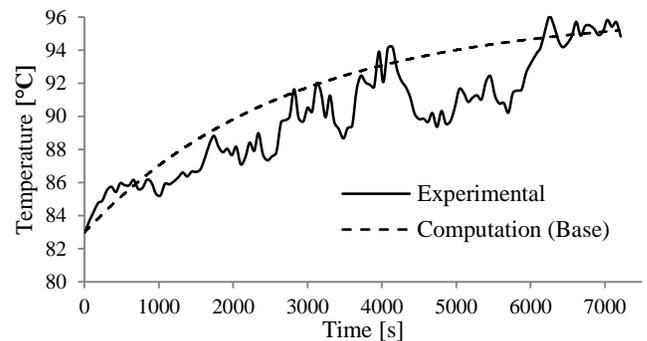
**Figure 7** Clutch housing air temperature variation during hill start vehicle test
