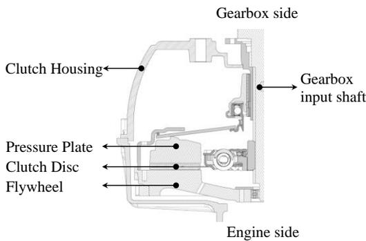
**Figure 1** Dry clutch system
