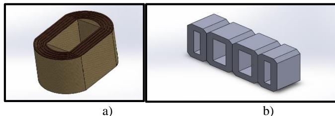
**Figure 2** CAD draw of the a) windings and b) silicon iron.
