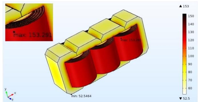
**Figure 13** Hot spot location for non-linear load configuration
