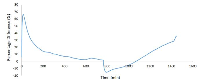
**Figure 12** Percentage of the residuals obtained from the comparison of numerical and experimental temperature values.
