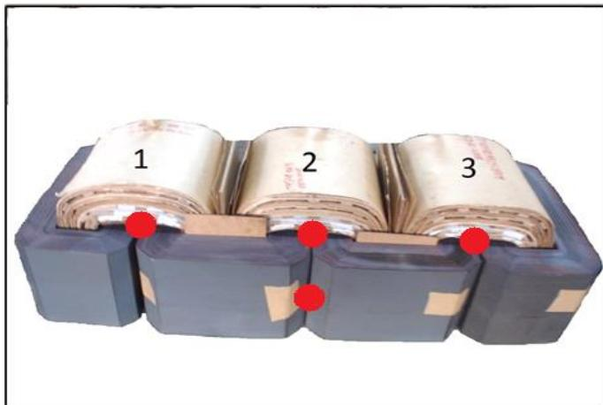
**Figure 7** Position of Temperature Sensors
