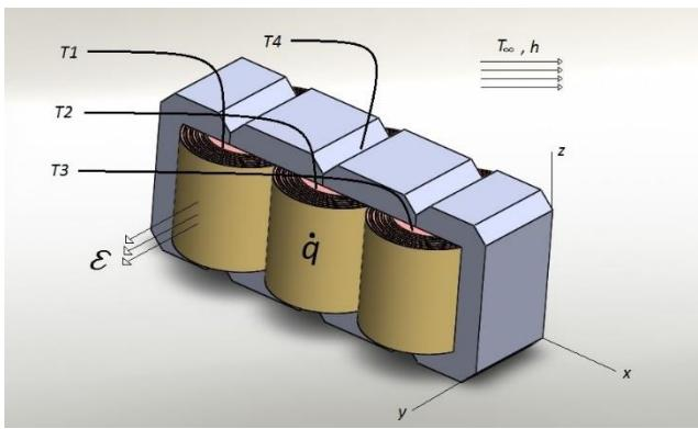
**Figure 1** Thermal model of the core.
