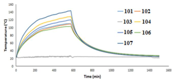
**Figure 8** Temporal evolutions of the experimental temperatures in the transformer with non-linear load.
