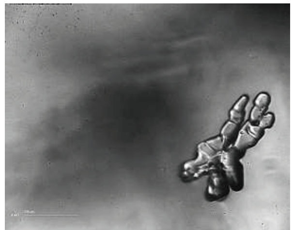
(f) Another ice crystal formed at -35 °C, with Re=16 , magnification of 60x
