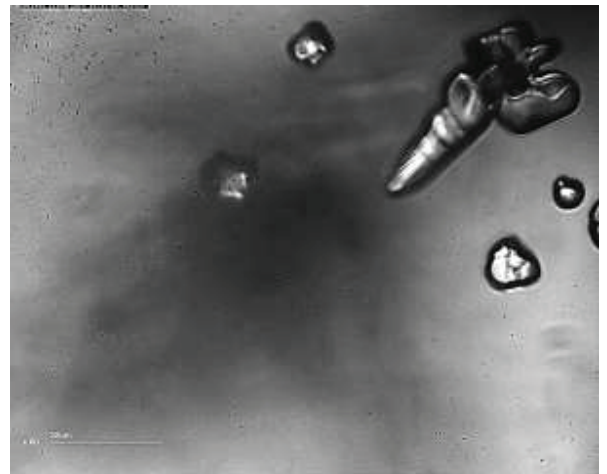
(e) Ice crystals formed at -35 °C, with Re=16 , magnification of 60x
