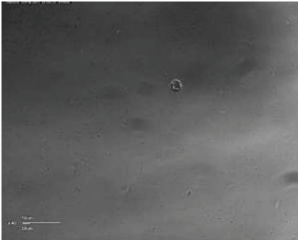
(a) An ice crystal formed at -15 °C, with Re=16 , magnification of 40x
