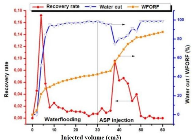
b) water cut, recovery rate and water flood oil recovery factor (WFORF) curves
