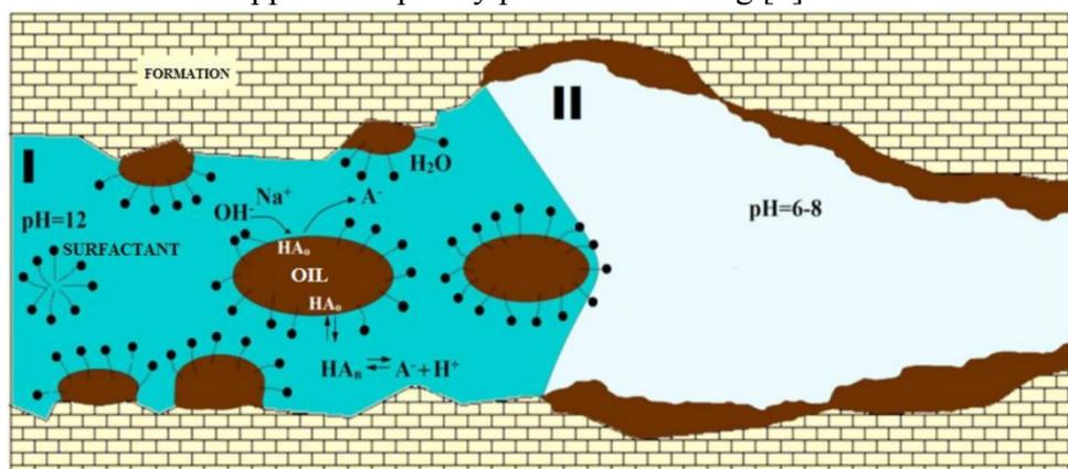
Figure 1. Mechanism of the ASP flooding of oil reservoir: I – alkali, II – neutral phase
