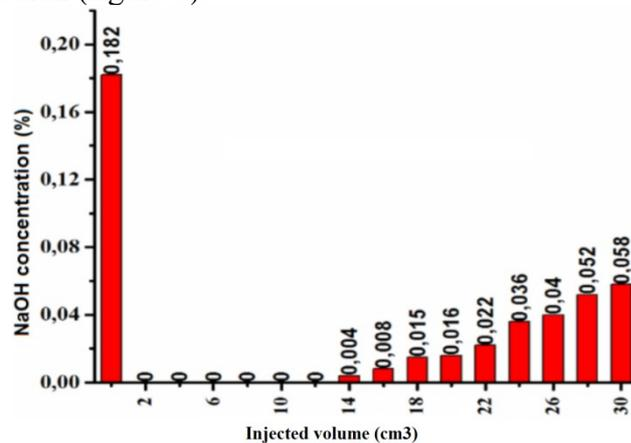
Figure 4. Change of NaOH concentration during agent filtration through physical model of the reservoir
