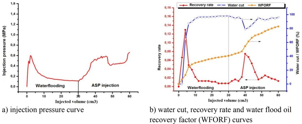
Figure 3. Sequential injection of water and aqueous solutions NaOH 0,2% + CRO-R-MAA(C13) 0,0125%
