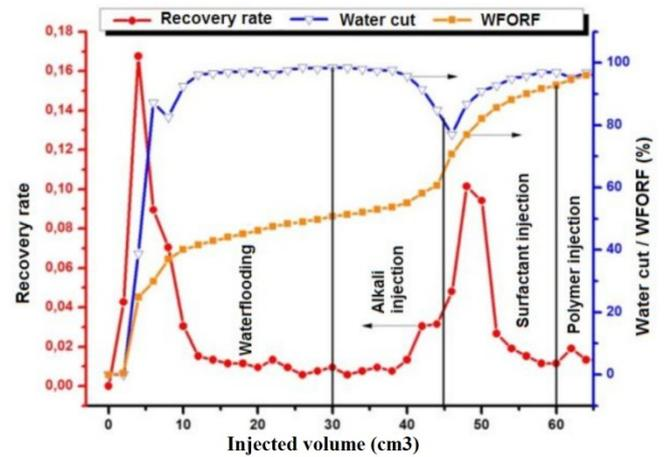
b) water cut, recovery rate and water flood oil recovery factor (WFORF) curves
