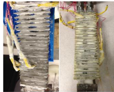
Figure 4 Silica gel type 3A with 3.3 wt% HEC binder coated heat exchanger.
