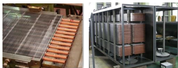
Figure 1 (a) Single module for adsorption bed and (b) stack of modules for adsorption bed construction.
