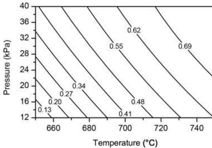
**Figure 10** The effect of temperature and pressure on the HFP mole fraction as determined by Meissner [6] in the second section of the horizontal reactor. The contour plot was generated using the response surface equations of Meissner [6] for HFP ( $Y_8$ ).
