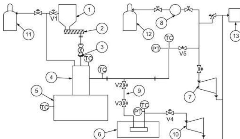
**Figure 1** Schematic layout of the continuous depolymerisation setup: (1) hopper, (2) screw feeder, (3) ball valve, (4) pyrolysis reactor, (5) furnace, (6) FTIR spectrometer, (7 and 10) vacuum pump, (8) diaphragm pump, (9) sampling tube, (11) inert gas cylinder, (12) holding cylinder, (13) vent.
