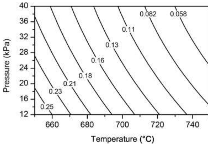
**Figure 7** The effect of temperature and pressure on the OFCB mole fraction as determined by Meissner [6] in the second section of the horizontal reactor. The contour plot was generated using the response surface equations of Meissner [6] for OFCB ( $Y_9$ ).
