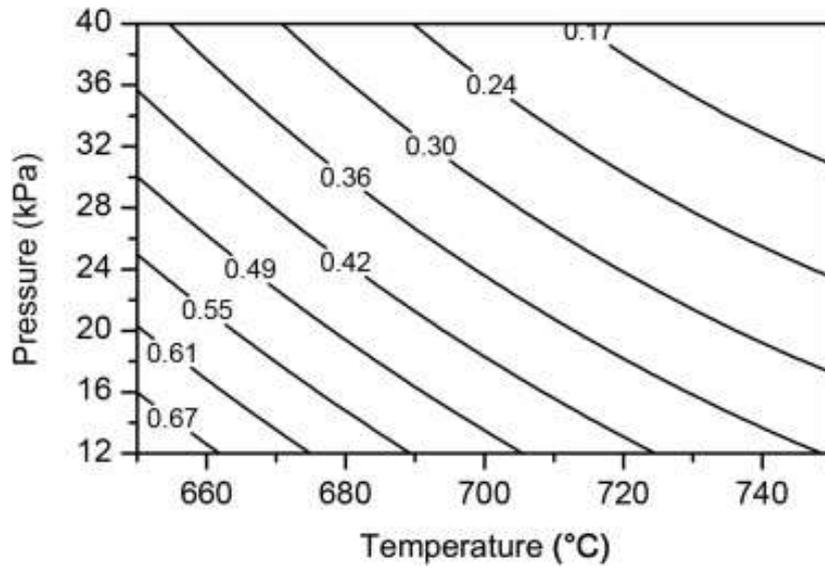
**Figure 3** The effect of temperature and pressure on the TFE mole fraction as determined by Meissner [6] in the first section of the horizontal reactor. The contour plot was generated using the response surface equations of Meissner [6] for TFE ( $Y_2$ ).
