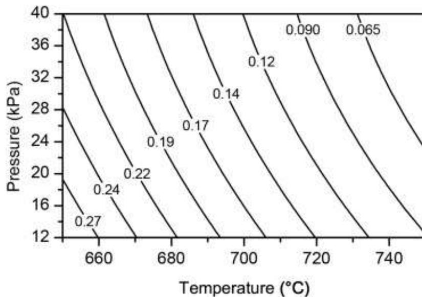
**Figure 6** The effect of temperature and pressure on the OFCB mole fraction as determined by Meissner [6] in the first section of the horizontal reactor. The contour plot was generated using the response surface equations of Meissner [6] for OFCB ( $Y_4$ ).
