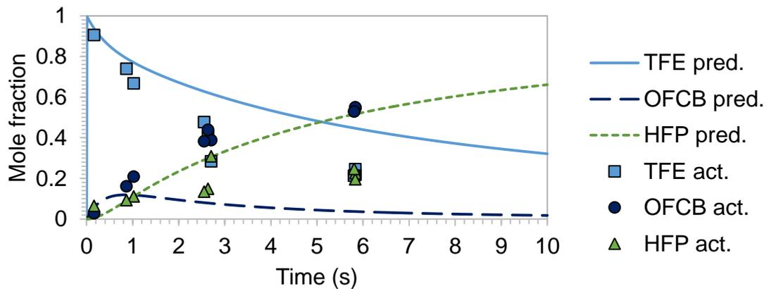
**Figure 13** The actual measured mole fractions of TFE, HFP, and OFCB and the predicted mole fractions determined via the differential equations as a function of residence time for a reaction temperature of 750 °C.
