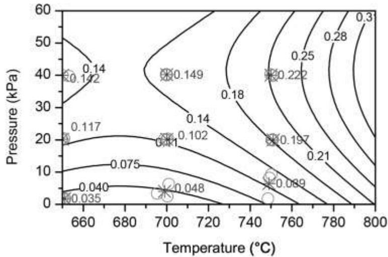
**Figure 8** The contour plot of the influence of temperature and pressure on the fractional distribution of HFP as calculated using equation 17. Data validation was achieved by including the actual experimental data points (O) and the averages calculated for each set which is denoted by a star.
