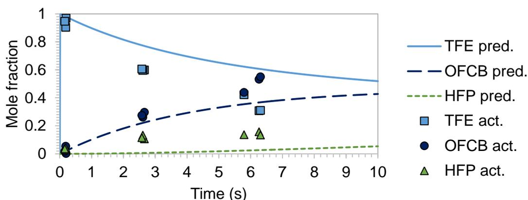
**Figure 11** The actual measured mole fractions of TFE, HFP, and OFCB and the predicted mole fractions determined via the differential equations as a function of residence time for a reaction temperature of 650 °C.
