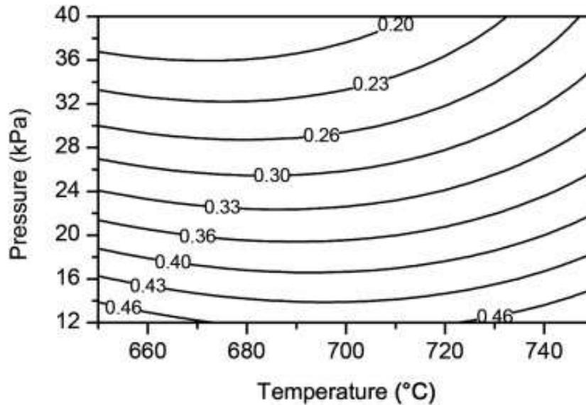
**Figure 4** The effect of temperature and pressure on the TFE mole fraction as determined by Meissner [6] in the second section of the horizontal reactor. The contour plot was generated using the response surface equations of Meissner [6] for TFE ( $Y_7$ ).
