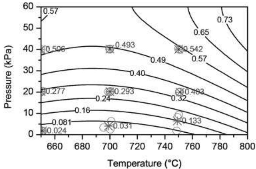
**Figure 5** The contour plot of the influence of temperature and pressure on the fractional distribution of OFCB as calculated using equation 16. Data validation was achieved by including the actual experimental data points (O) and the averages calculated for each set which is denoted by a star.
