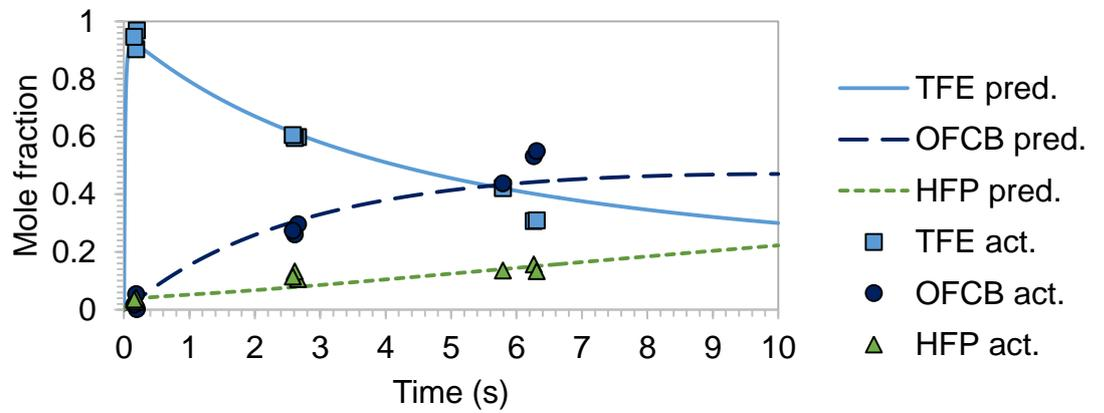
**Figure 14** The determined formation rates of TFE, HFP, and OFCB over time compared to the actual product fractions at a temperature of 650 °C.
