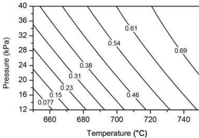
**Figure 9** The effect of temperature and pressure on the HFP mole fraction as determined by Meissner [6] in the first section of the horizontal reactor. The contour plot was generated using the response surface equations of Meissner [6] for HFP ( $Y_3$ ).
