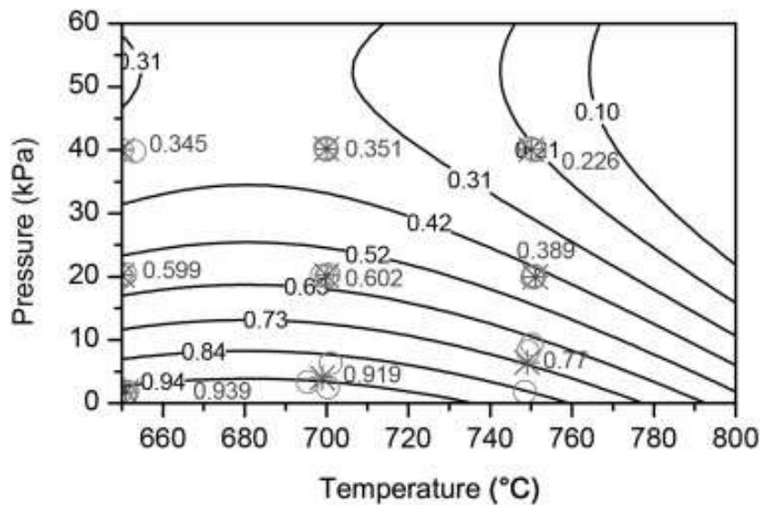
**Figure 2** The contour plot of the influence of temperature and pressure on the fractional distribution of TFE as calculated using equation 15. Data validation was achieved by including the actual experimental data points (O) and the averages calculated for each set which is denoted by a star.
