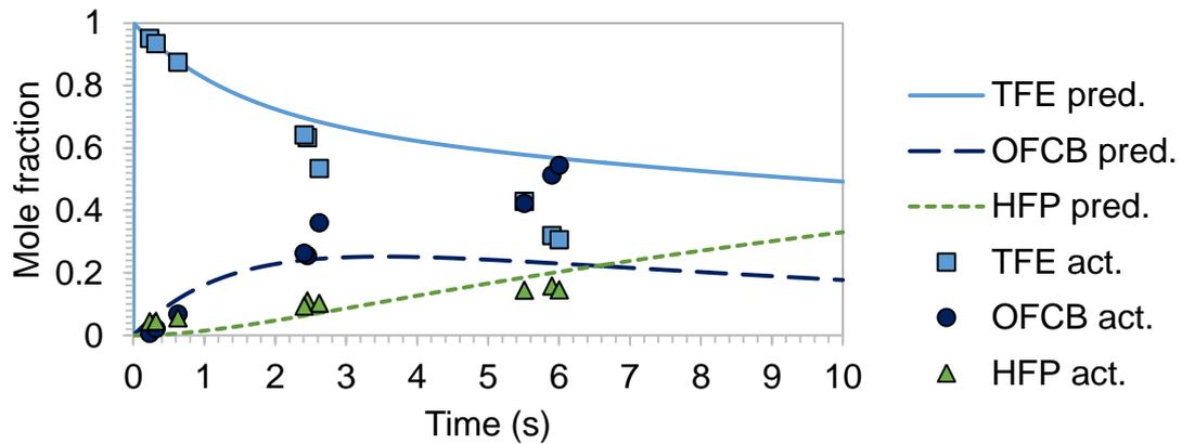
**Figure 12** The actual measured mole fractions of TFE, HFP, and OFCB and the predicted mole fractions determined via the differential equations as a function of residence time for a reaction temperature of 700 °C.
