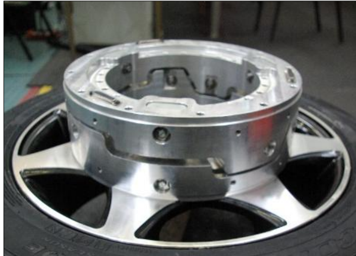
Figure 2.5 - Wheel Force Transducer (WFT) mounted onto the sample tyre rim
