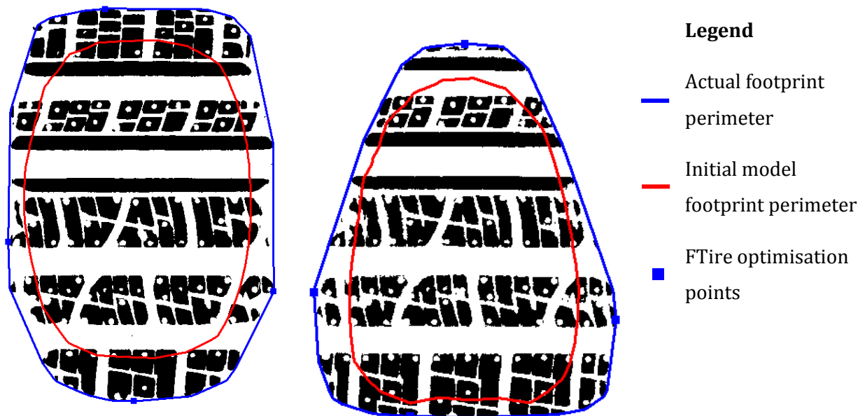
Figure 4.8 - Initial validation of footprints at 50% of the LI: 0° camber (Left), -4° camber (Right)
