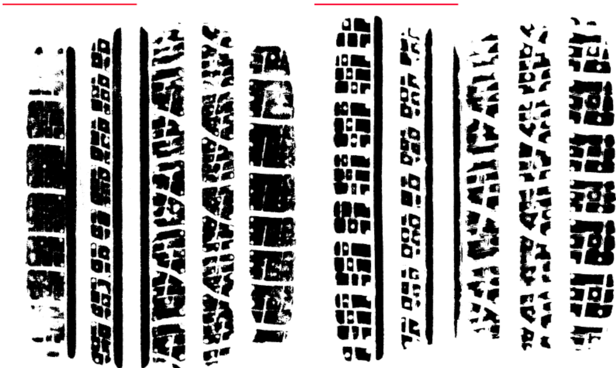
Figure 5.5 - Footprint comparison at 0° camber at 100% of the LI - New Tyre (Left), Aged Tyre (Right)
