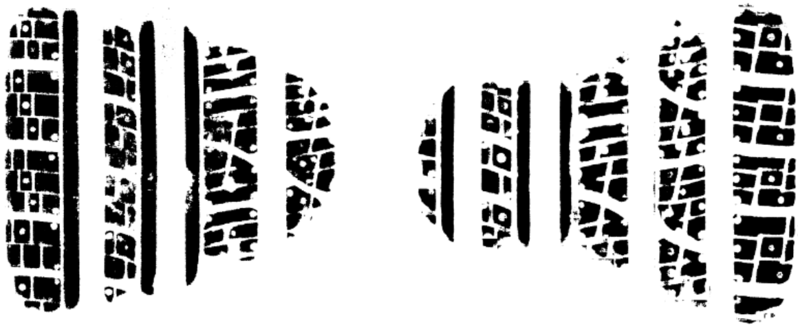
Figure 5.9 - Footprint comparison of 2.5 Bar Inflation at 4° camber at 50 % of the LI - New Tyre (Left) and Aged Tyre (Right)
