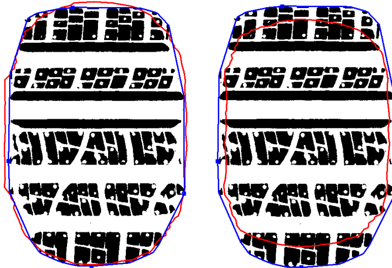
Figure 6.23 - Changes in the footprint at 0° camber after model update of mass and tread depth - Left is the original model, Right is the updated model
