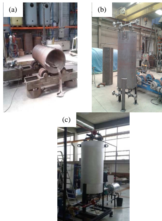
Figure 3 Heat exchanger: a) a helical coil; b) final assembly of the component; c) insulated and installed component in the installation in the laboratory
