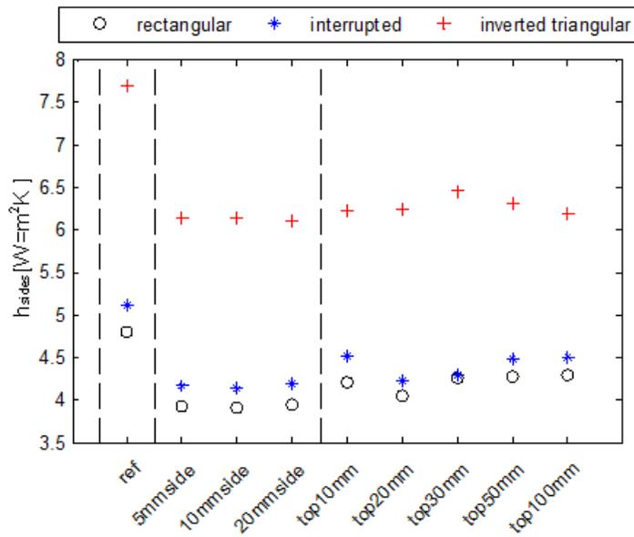
**Figure 4.** Dependency of the heat transfer coefficient on the fluid domain at the sides of the fin row ( $h_{sides}$ )
