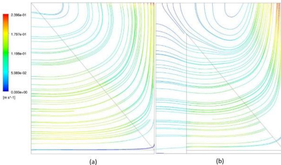
**Figure 9.** Velocity contour plot and streamlines in the middle of the inverted triangular fin row, (a) without added fluid domain ('Mesh-ref'), (b) with 20 mm of fluid domain added at the sides and top ('Mesh-top20mm', right side: symmetry plane).
