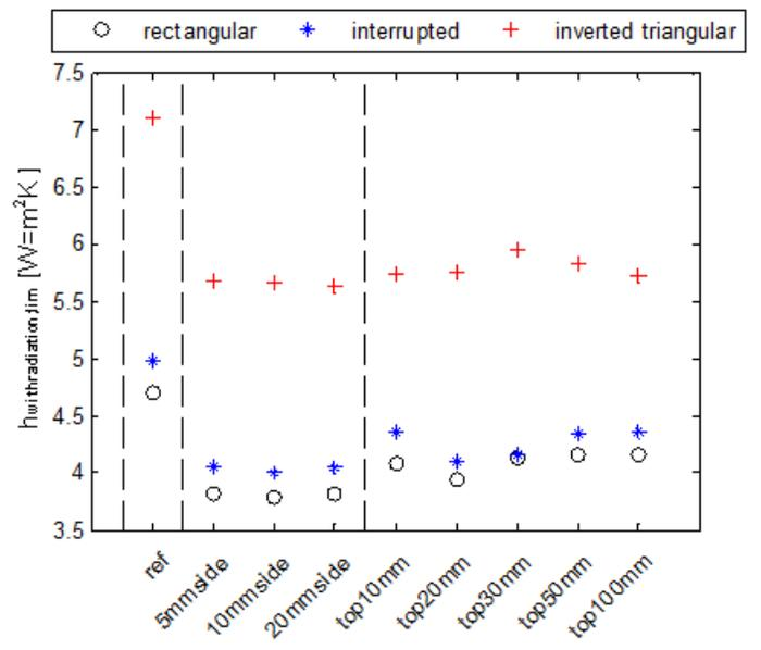
**Figure 7.** Dependency of the heat transfer coefficient on the fluid domain, taking an area-average of  $h_{sides}$  and  $h_{bottom}$  into account ( $h_{with\ radiation, itm}$ ).
