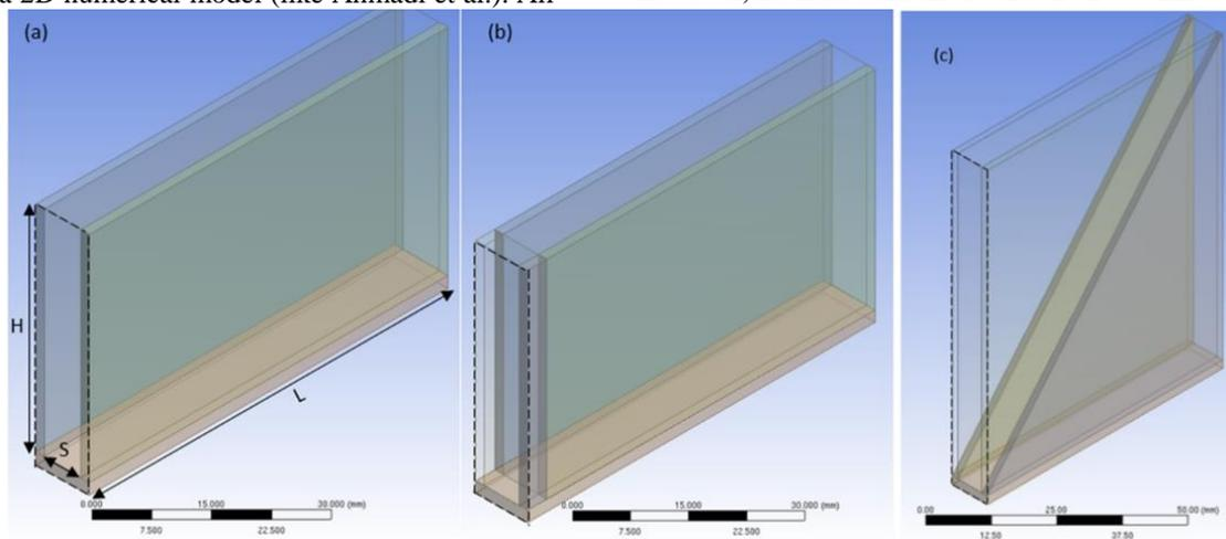
**Figure 1.** Illustration of the used fin shapes in this work. (a) rectangular fin, (b) interrupted rectangular fin, (c) inverted triangular shape. Dashed line indicates the symmetry plane.
