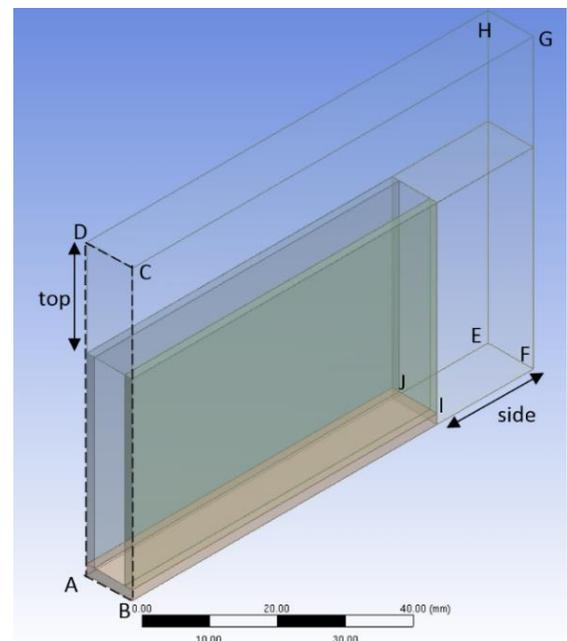
Figure 3. Illustration of the boundary conditions in case of a rectangular fin row ('Mesh-top20mm')
