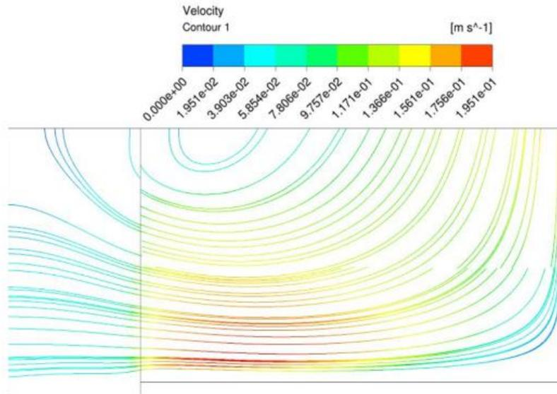
**Figure 8.** Velocity contour plot and streamlines in the middle of the rectangular fin row with 20 mm of fluid domain added at the sides ('Mesh-20mmside', right side: symmetry plane)
