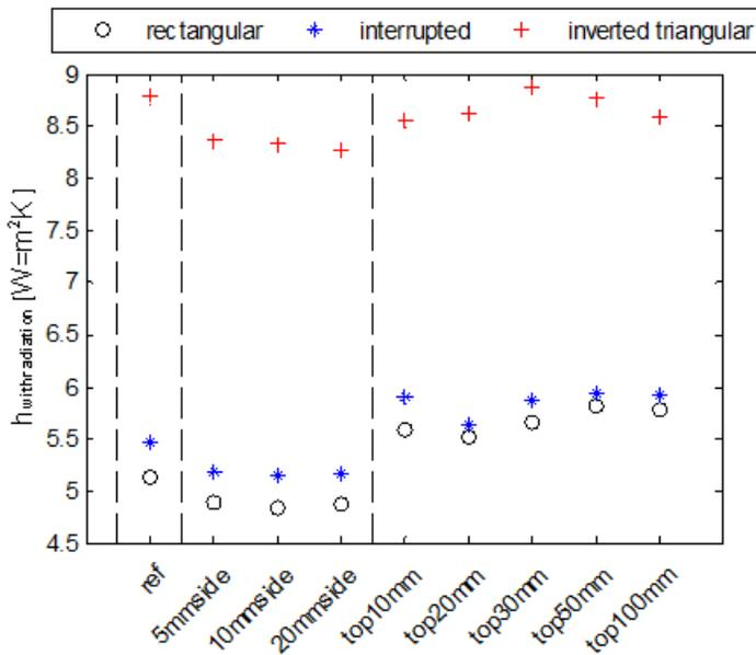
**Figure 6.** Dependency of the heat transfer coefficient on the fluid domain, taken all the available surfaces into account ( $h_{with\ radiation}$ ).
