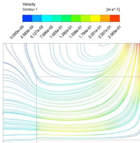
**Figure 10.** Velocity contour plot and streamlines in the middle of the rectangular fin row with 20 mm of fluid domain added at the sides and top ('Mesh-top20mm', right side: symmetry plane)
