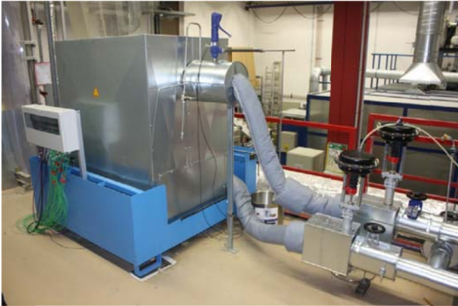
Figure 1 Experimental set-up of flat plate latent heat storage at DLR [9].
