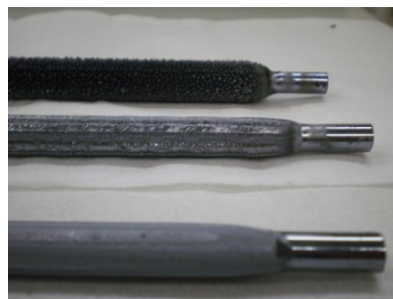
Figure 2 Polysilicon rods after deposition processes conducted in the laboratory Siemens reactor at 1000 °C (bottom), 1100 °C (middle) and 1150 °C (top)
