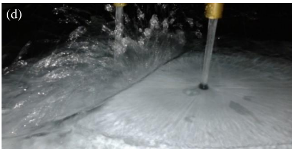
Figure 3 (a) Two far-distant impinging jets indicating no jump interactions. (b) Two jets spaced at a critical distance (c) formation of upwash (d) Upwash fountain flow.
