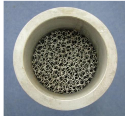
Figure 2 Photograph showing metal foam brazed to inside surface of the test section
