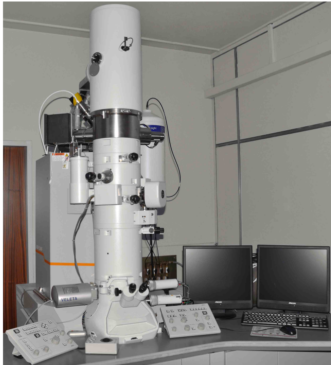
Figure 1.10 Transmission Electron Microscope. The Joel JEM 2100F Field Emission Electron Microscope of the Laboratory of Microscopy and Microanalysis of the University of Pretoria. Photograph: Tanya Marie Downing.
