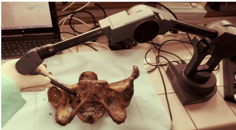
Figure 3.14: 3DXL MicroScribe® digitiser pointing to a bony landmark
