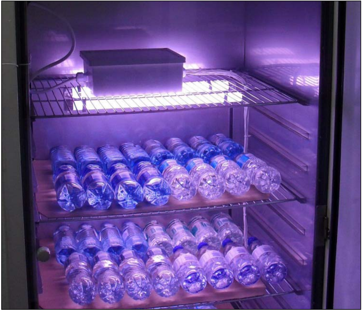
Figure 3.8: Incubator setup for the exposure of bottled water samples to simulated sunlight
