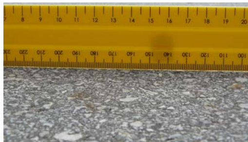
FIGURE 6 Continuously Graded Asphalt with 1/3 rd octave sound level spectrum (dBA) at 10m. Traffic flow: 80 km/h, 560 veh/h, 15% heavy duty veh
