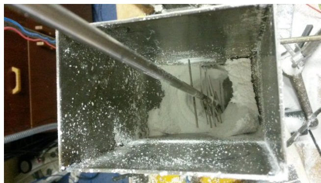
Figure 43: System with the stirrer inserted inside of the hopper. One can see the heavily compacted PTFE resulting from over stirring the particles.
