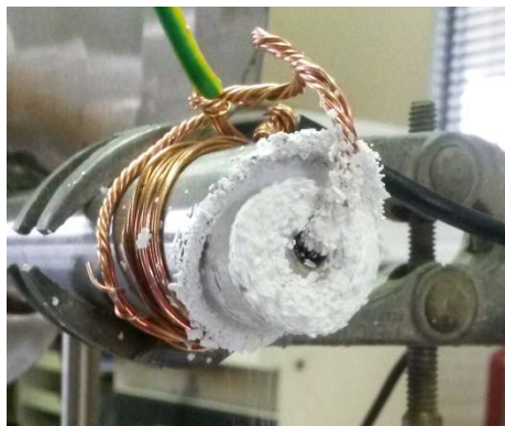
Figure 30: Static build-up at the screw exit.
