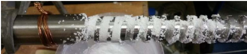
Figure 29: Severe screw clogging
