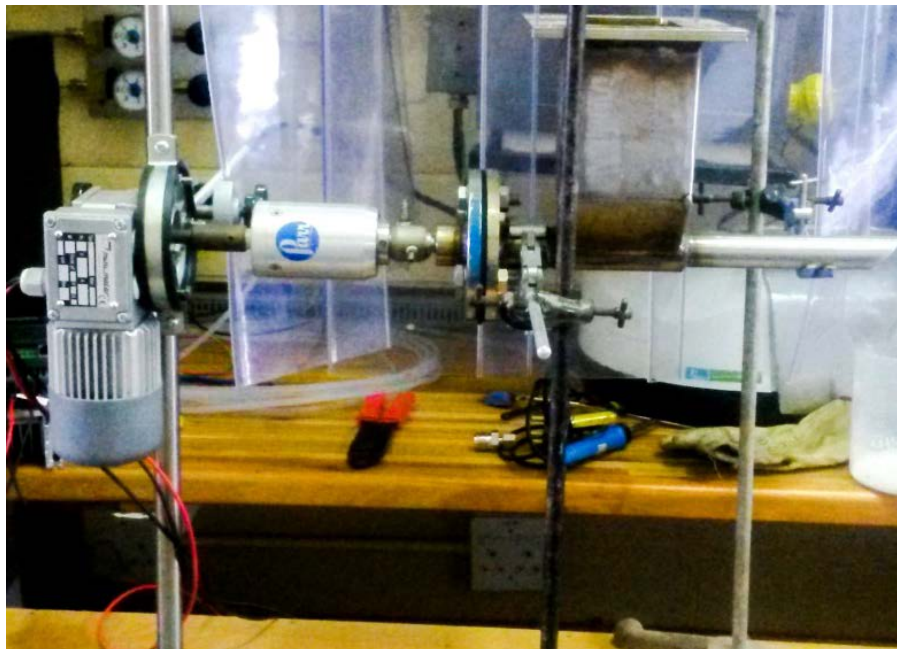
Figure 28: Actual testing feeder system.
