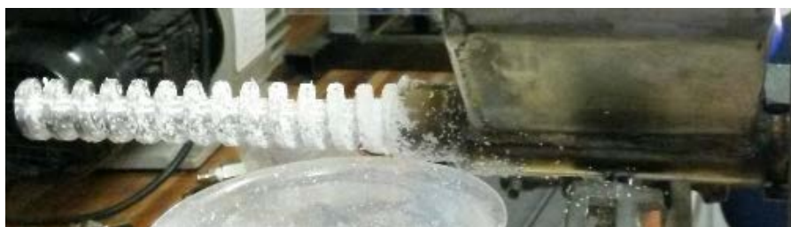
Figure 31: The testing system with shortened screw feed tube.
