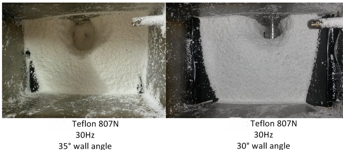
Figure 34: Rat-hole formation experienced in the hopper at two different hopper angles for a motor speed of 22 rpm (30 Hz).
