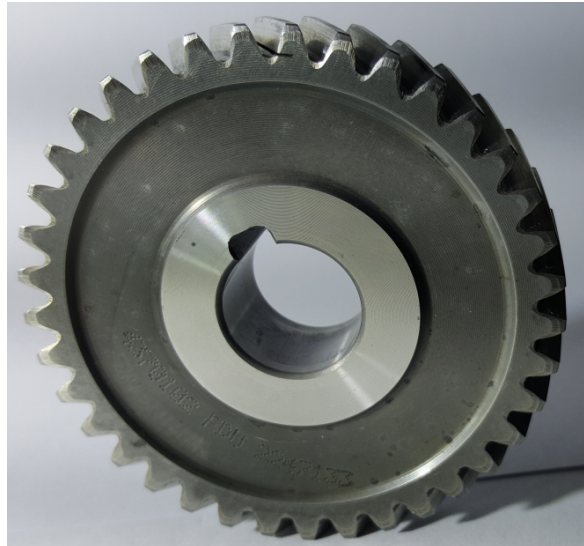
Figure 2.7: The damaged gear of the first experiment.
