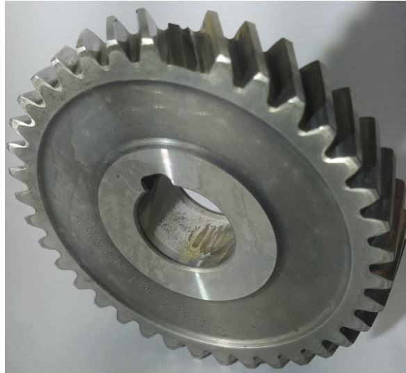
Figure 2.9: The damaged gear in figure 2.7 after more than 45 days of experiments.
