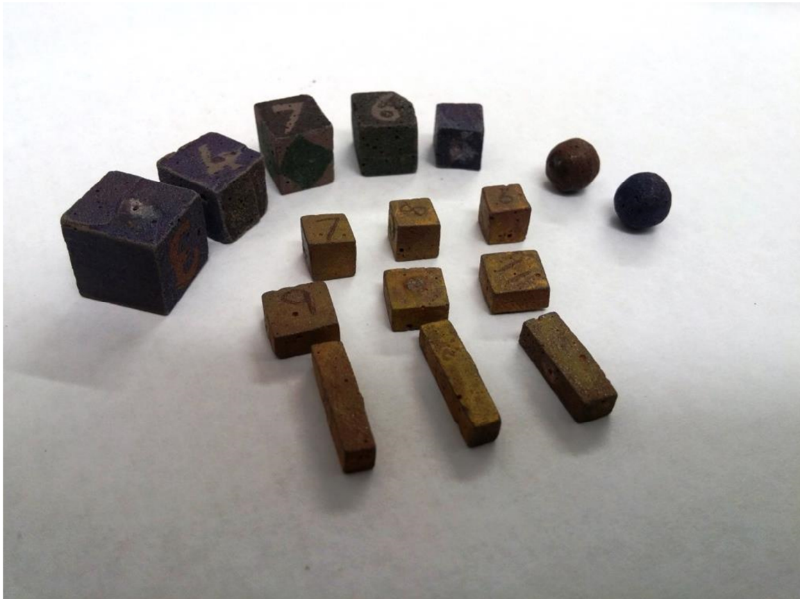
Figure 5-3 Photo of the artificial tracers used for the PEPT jiggling experiments
