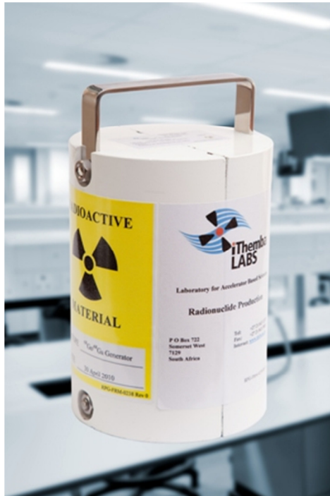
Figure 4-5 Gallium 68 generator ( http://s15.a2zinc.net , 2014)
