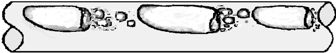
Figure 2.5: Slug flow pattern
