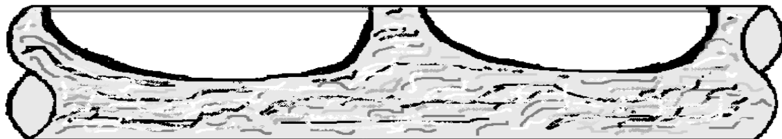
Figure 2.6: Plug flow pattern
