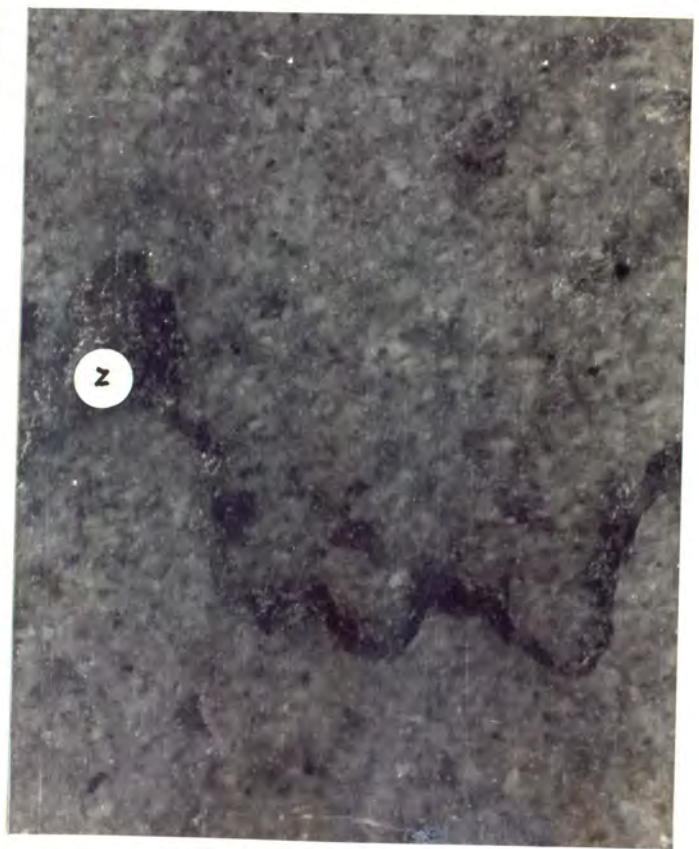
A shows four stylolites in the processes of formation (Mag.x4). B shows typical well-developed stylolite (X Polars Mag.x4). C stylolite with microfracture Y. D stylolite with cross-cutting channel z represents a weak point (Mag.x8).
