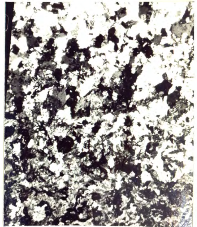
1. A study of grain boundaries of crystals. It also shows the inclusions which give a clouding effect in orthoclase and plagioclase (x 100, crossed nicols). B. The textural nature of the arkosite (x 60, crossed nicols). C. The recrystallised arkosite with considerable interpenetration near pocket haloes (x 60, crossed nicols). D. Arkosite in the bottom left becomes more quartzitic in the bleached halo area, top right (x 15 crossed nicols).
