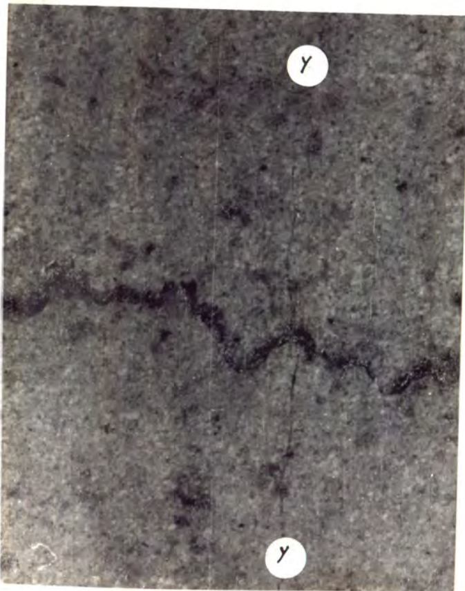
A shows four stylolites in the processes of formation (Mag.x4). B shows typical well-developed stylolite (X Polars Mag.x4). C stylolite with microfracture Y. D stylolite with cross-cutting channel z represents a weak point (Mag.x8).
