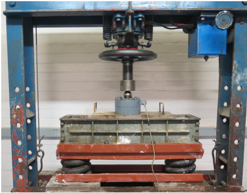
Figure 3.8: The press used for consolidation of the clay.
