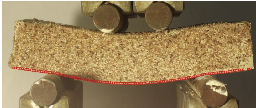
Figure 3.19: Tracking the edge of the beam using DIC.
