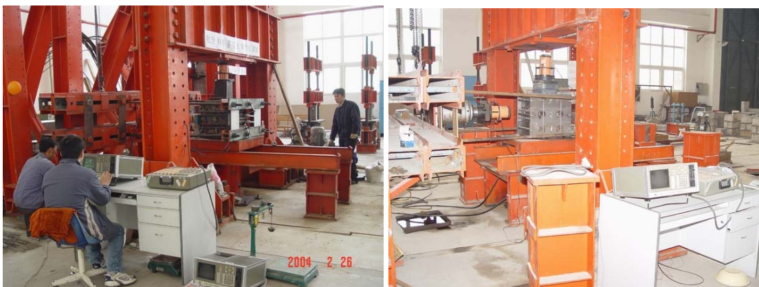
Figure 1. Shearing test equipment.
