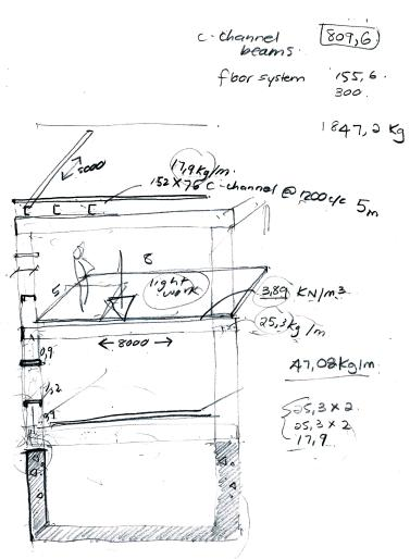
Figure 7.12: Sizing of steel structure. (Author, 2016)
