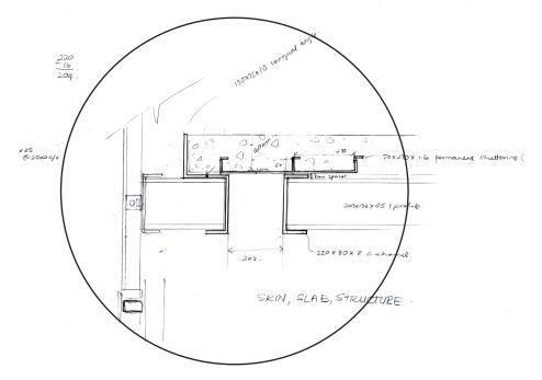
Figure 7.11: Bondlok fixed to I-profile joist (Author, 2016)
