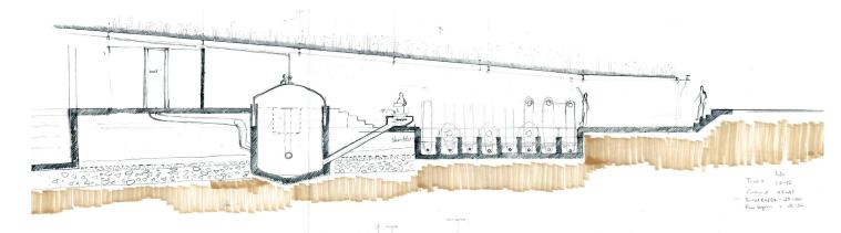
Figure 7.9: Planted roof and tapered gabion walls. (Author,2016)
