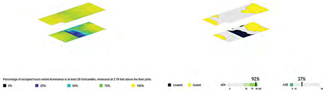
Figure 78. Daylighting iterations and investigations through detailed section (Author 2016).
