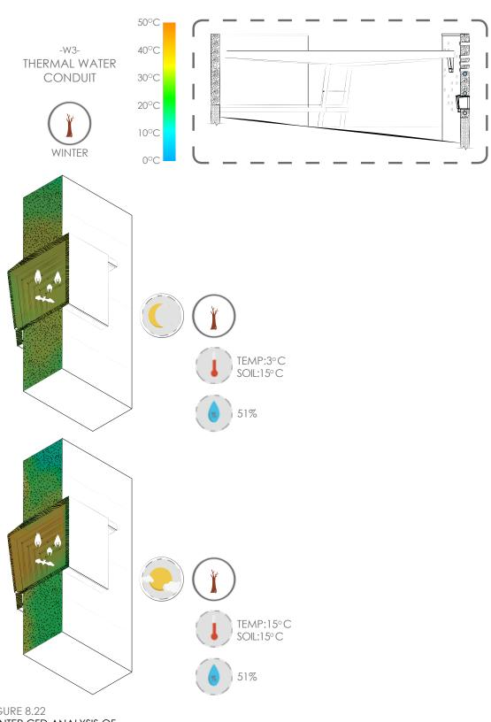
FIGURE 8.22 WINTER CFD ANALYSIS OF THERMAL WATER CONDUIT (Author, 2015)
