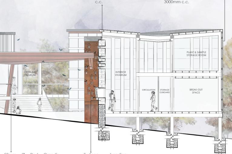
50mm Ø Red Grandis Saligna circular grabrail @ min 900mm fixed with epoxy to 10mm galvanised steel pin connection, fixed to 25mm Ø galvanised steel post, welded to 50x50mm steel baseplate, bolted to 300x100mm laminated SA pine bearer @ 3000mm c.c.
