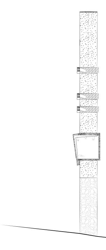
FIGURE 9.12 VIVARIUM CHIROPTERA ROOST STABILISED EARTH WALL SECTION NOT TO SCALE (Author, 2016)
