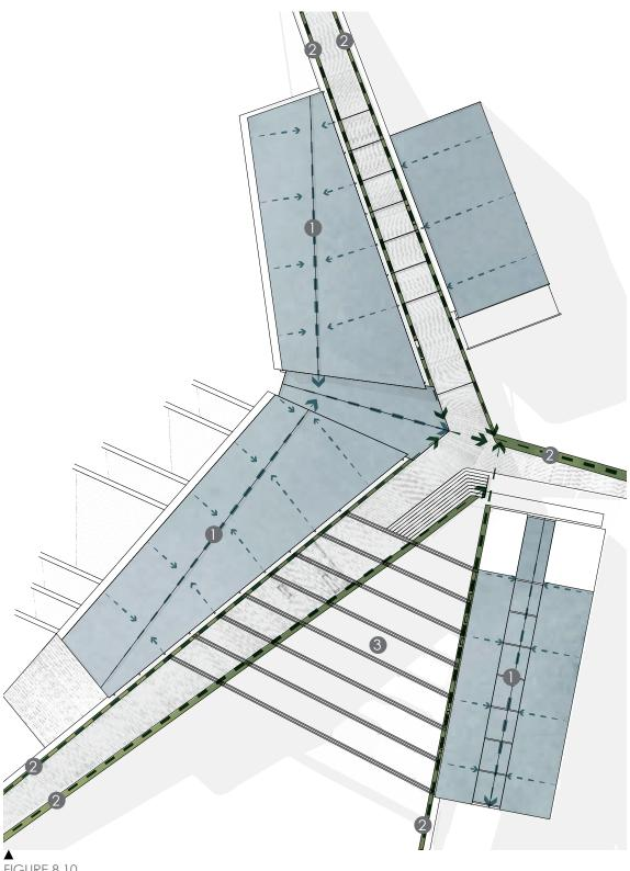
FIGURE 8.10 VIVARIUM ROOF & DRAINAGE PLAN (Author, 2016)
