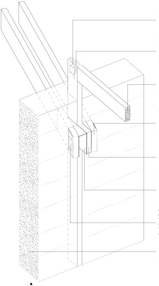
GRAPHITE-GREY POWDER COATED 300x150x3mm STEEL WALL PLATE BOLTED TO LAMI-NATED TIMBER BEAM WITH 4x12mm Ø GRADE 2 BOLTS
