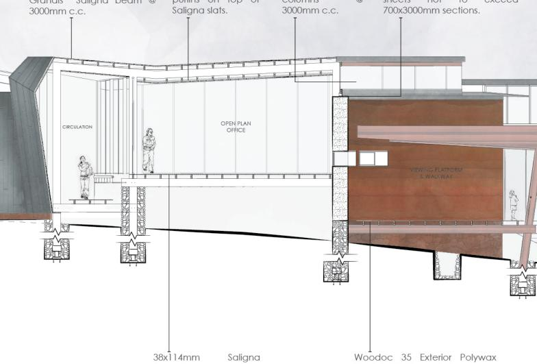
38x114mm Saligna tongue and groove boards conceal fixed to 150x50mm SA pine floor joists @ 600mm c.c. screwed to 300x100mm laminated SA pine bearer @ 3000mm c.c.
