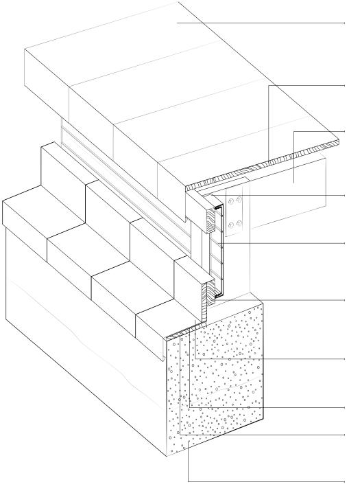
PROTECT GRAPHITE-GREY 0.8mm RHEINZINK-FLAT LOCK TILE SYSTEM OR SIMILAR APPROVED @ 300mm c.c., ON AIR-Z STRUCTURED MAT OR SIMILAR APPROVED, FIXED TO PLYWOOD BOARDING
