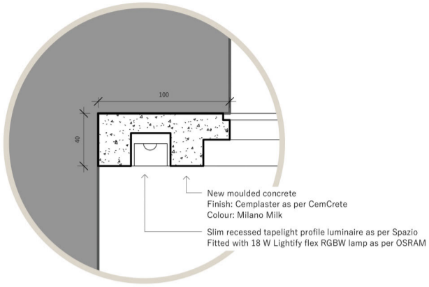
010 LIGHT STRIP DETAIL SCALE 1:5
