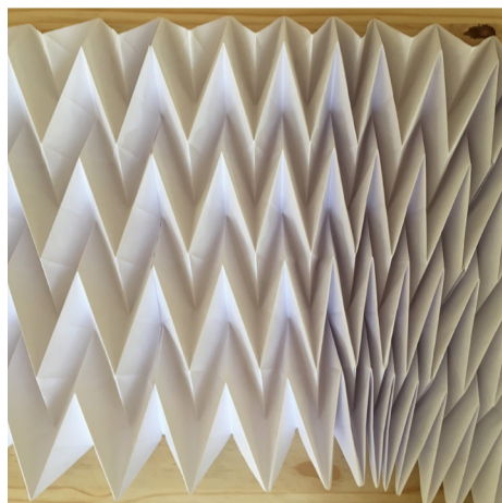
Figure 5.3.12 Collapsed multiple v-fold (Author. 2016)
