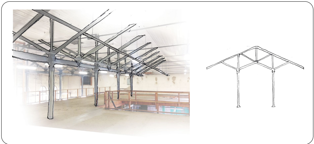
Figure 4.8: Exposed structural system - Allows for large open-plan adaptable spaces that are not dependent on perimeter walls for structural integrity.
