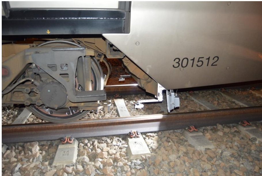
Figure 3.33: Side View of Cameras and Spotlights Installed in front of Wheel 1 and Wheel 8 on Axle 1 of DMOS B on Ballasted Track
