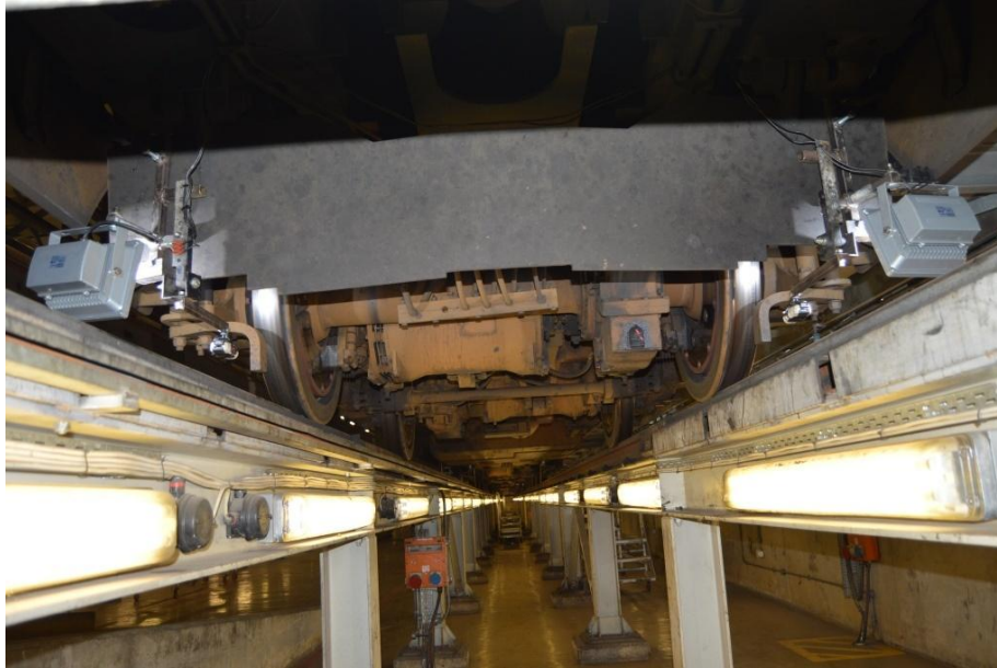
Figure 3.31: View from under the Train of Cameras and Spotlights Installed in front of Wheel 1 and Wheel 8 on Axle 1 of DMOS B on the Workshop Maintenance Line
