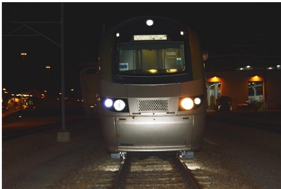
Figure 3.34: Front View of Cameras and Spotlights Installed in front of Wheel 1 and Wheel 8 on Axle 1 of DMOS B on Ballasted Track
