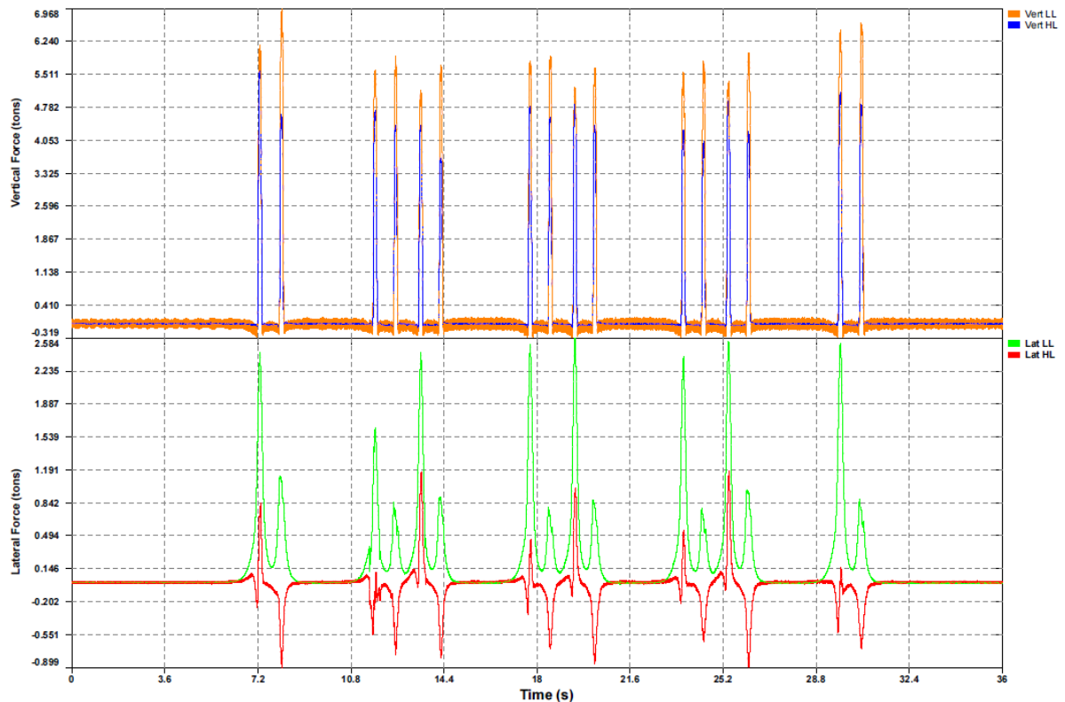
Figure 3.40: Vertical and Lateral Rail Forces After Tamping (10km/h, S2 Up)
