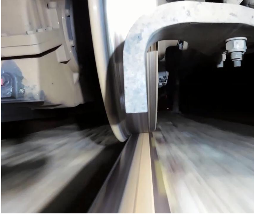
Figure 3.3: High Leg Contact to the Gauge Side of the Rail in the Experimental Curve
