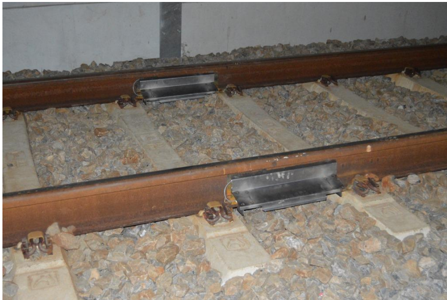
Figure 3.25: Encapsulated Strain Gauges Covered by Stainless Steel Cover Plates
