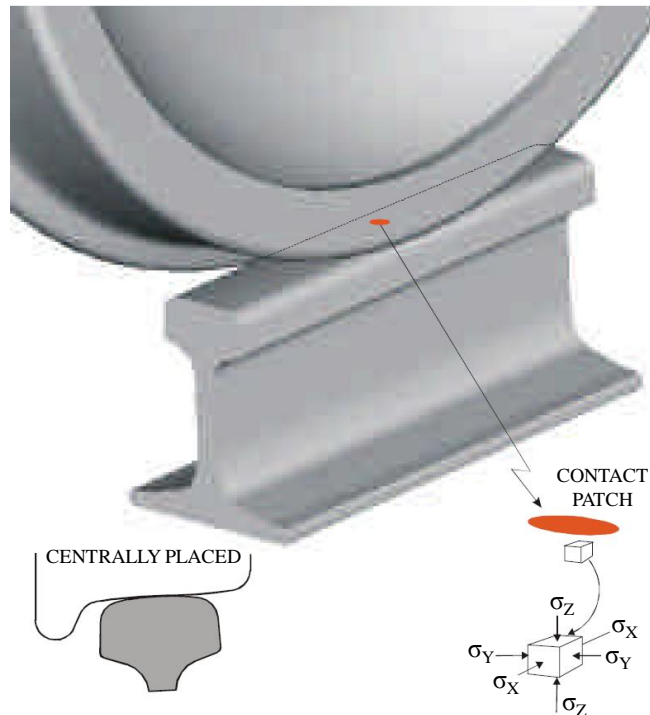
Figure 2.11: Contact Between Wheel and Rail: Wheel Centrally Placed on the Track, from Harris, et al. (2001)
