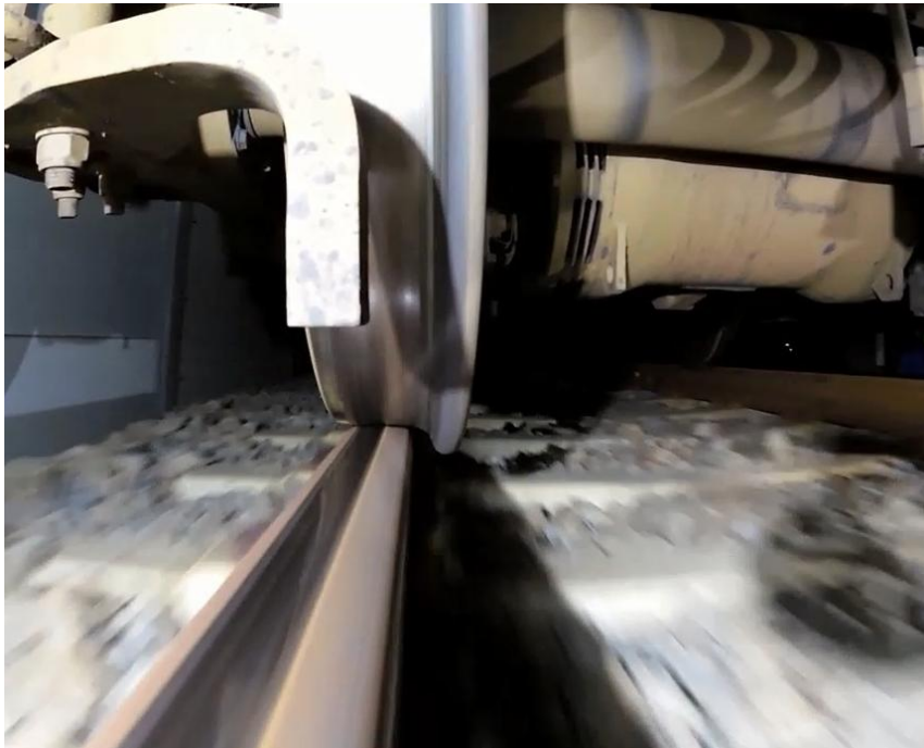
Figure 3.4: Low Leg Contact to the Field Side of the Rail in the Experimental Curve
