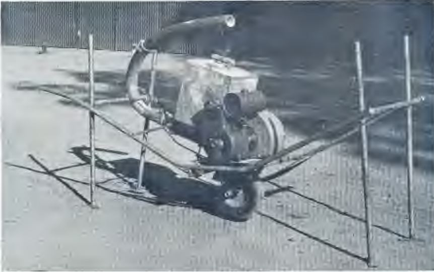
FIG. 9.—Mechanical duster mounted on single wheel.
