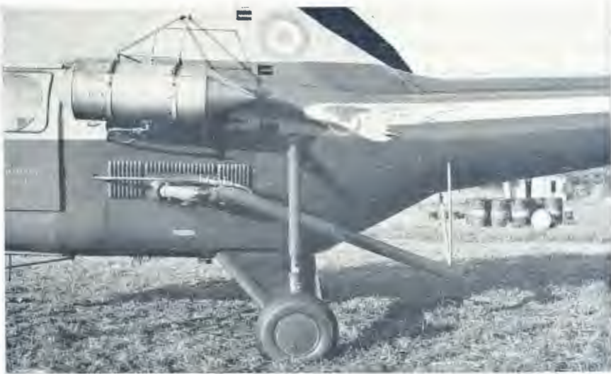
FIG. 8.—Sikorsky S51 helicopter showing modified exhaust stack and point of entry of insecticidal solution.
