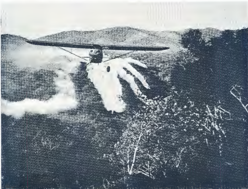
FIG. 6 (b)—Piper cruisers applying smoke. Forced feeding insecticidal solutions enables columns to be laid in all flying positions.
