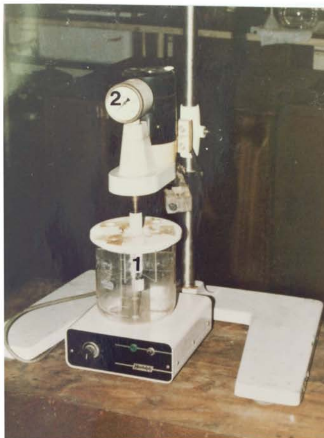
PICTURE 7 Apparatuses used for mass loss turbulence tests
