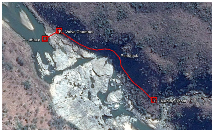
Figure 7.2: Intake and penstock location and layout of Nnodekhling-Shayiwe (Bonthuys, 2015)
