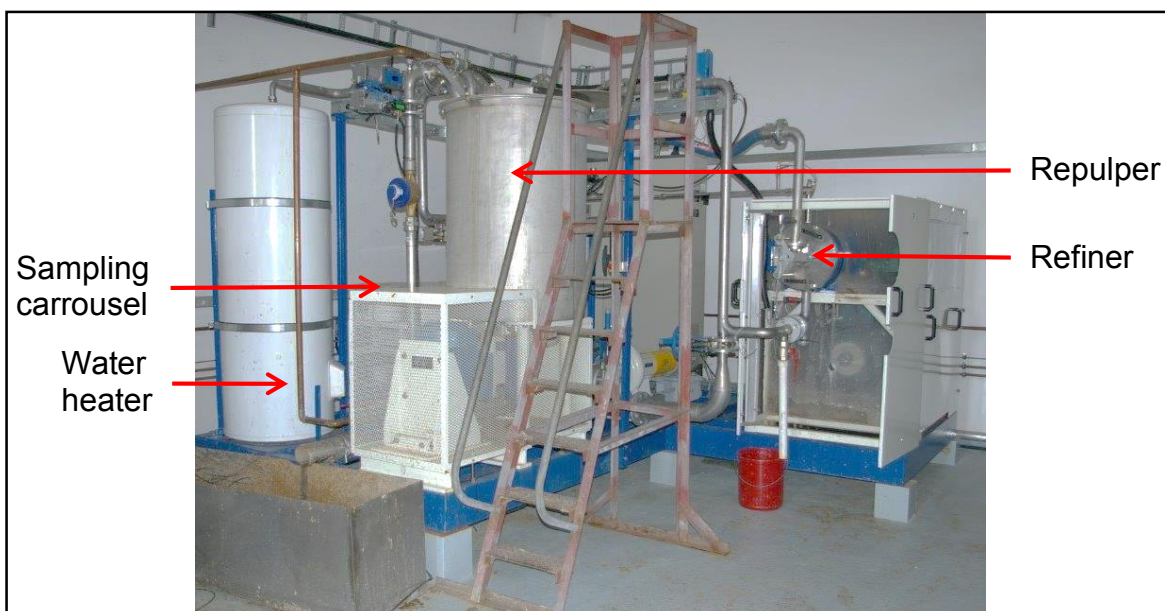
Figure 2-2: The pilot refiner circuit at the Sappi Technology Centre (Pretoria).
