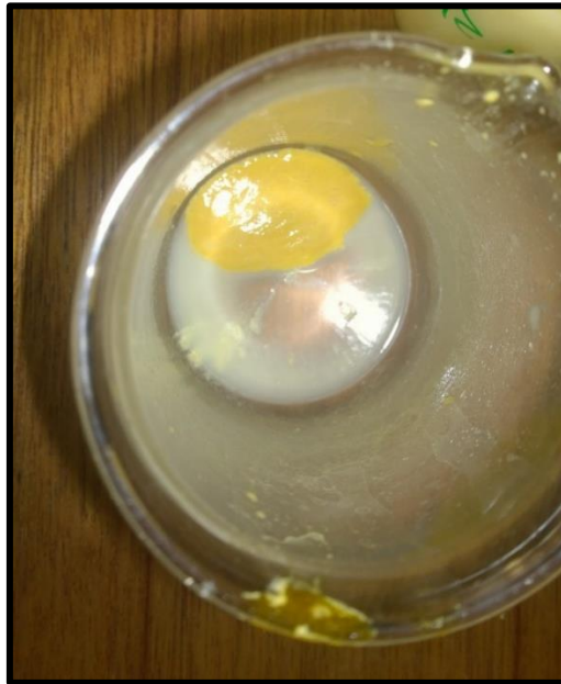
Figure 4-3: Precipitated zein and micro-particles formed after phase separation in the wintergreen oil-zein system.
