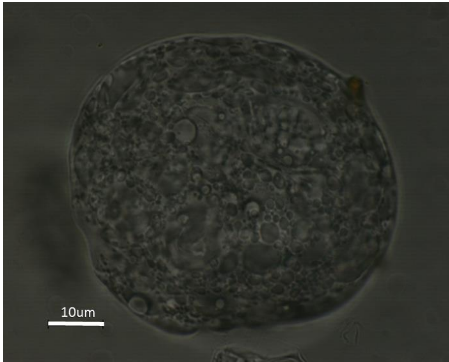
Figure 4-20: Close-up image of a large micro-particle of the geraniol-to-zein 3:1 system.
