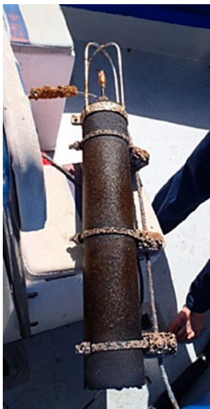
FIGURE 4 First retrieval and service (after deployment on the 2nd of September 2013) of the loggerhead DSG-Ocean on 1st October 2013. PHOTO CREDIT HARRY STONE
