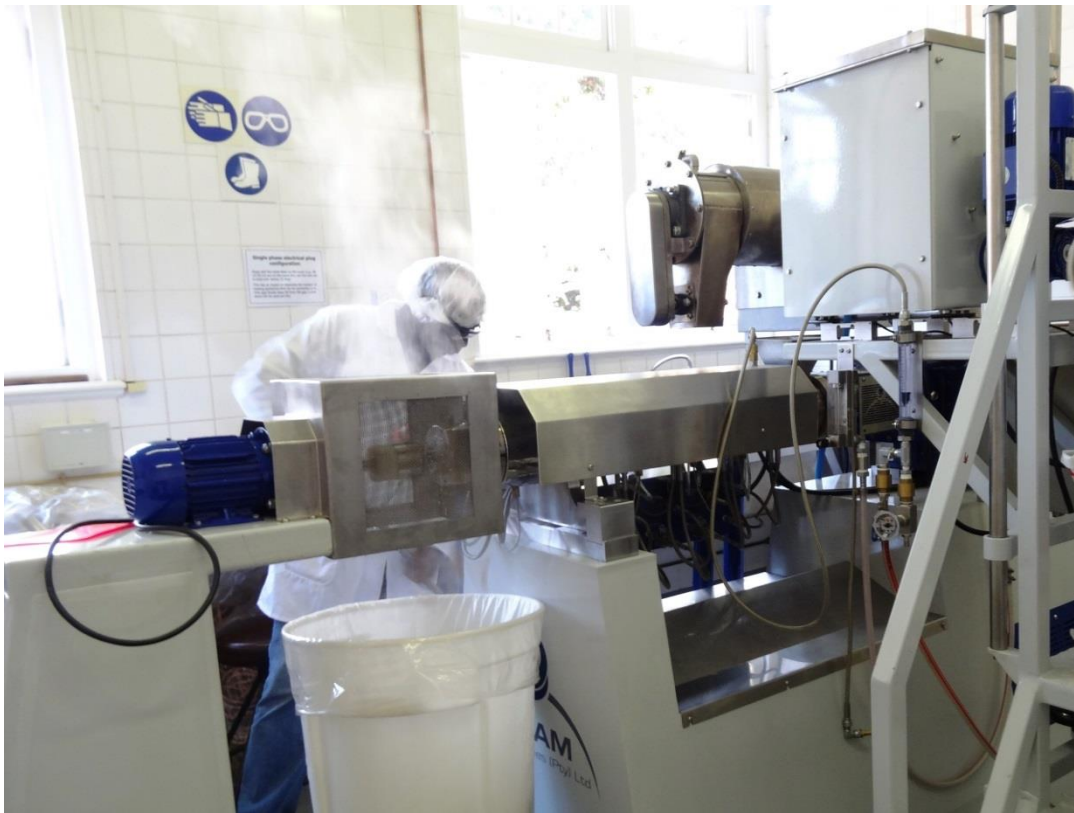
Figure 2.2: Type of extruder similar to the TX 32 twin screw, co-rotating extruder (CFAM Technologies, Potchefstroom, South Africa) used in the study. Image courtesy: Prof J. R. N. Taylor.
