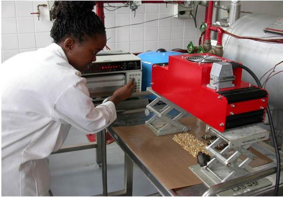
Figure 4.3: Table top microniser (Technilamp, Johannesburg) which was used in the study. Images courtesy: Prof J. R. N. Taylor.
