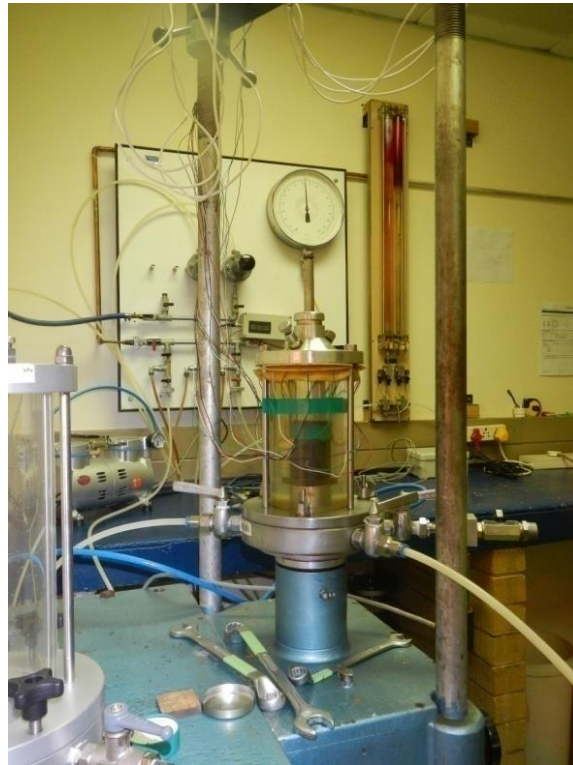
Figure 21: Pore pressure transducers being saturated and calibrated in the modified triaxial cell mentioned in Le Roux (2013).
