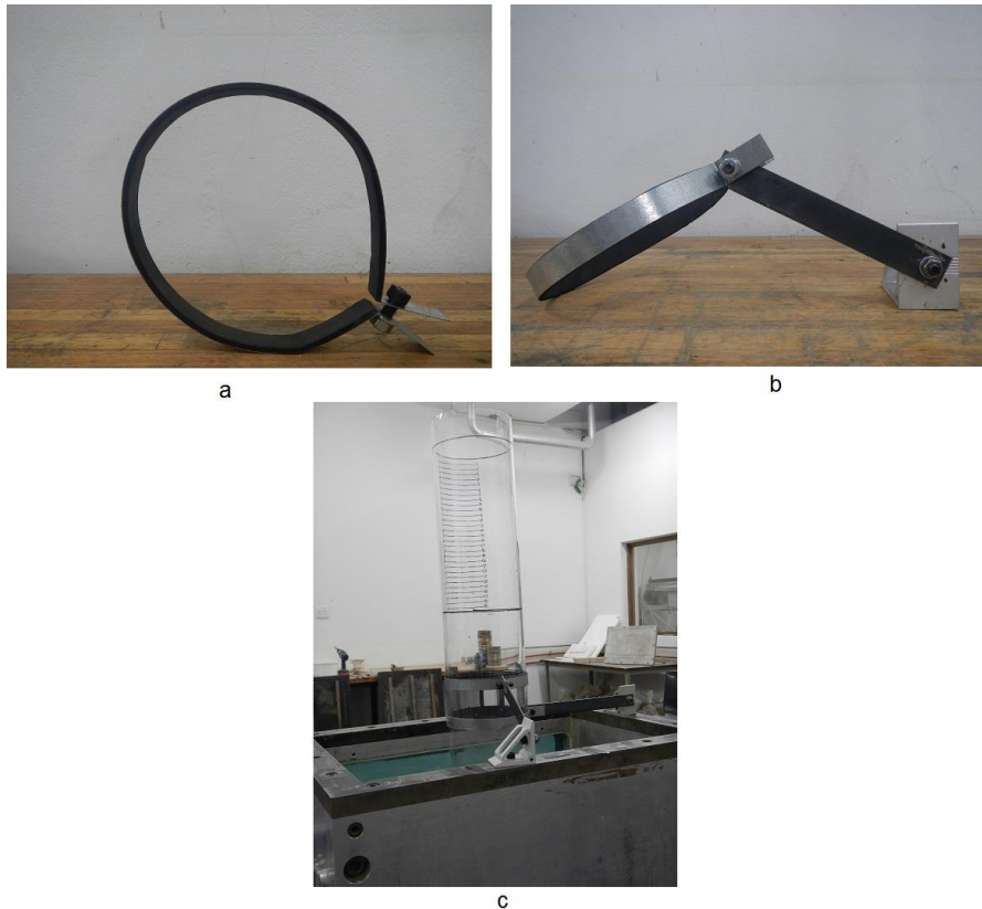
Figure 15: (a) The foam lined ring clamp that was used to fix the support bars to the cylinder. (b) The support bar connected to the ring clamp and the 90° bracket. (c) The support system fixed to the strong box collar and attached to the cylinder, with the support bars at 90° from each other.
