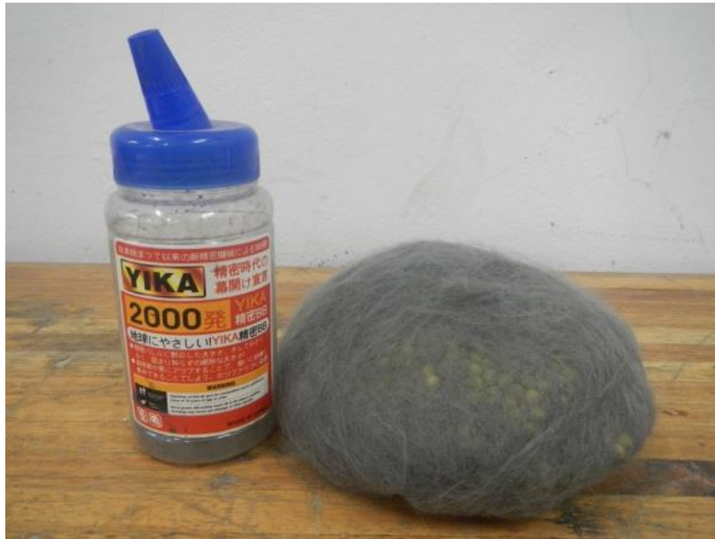
Figure 16: The 6 mm BB bullets enclosed in the A4 Bidim to form the filter.
