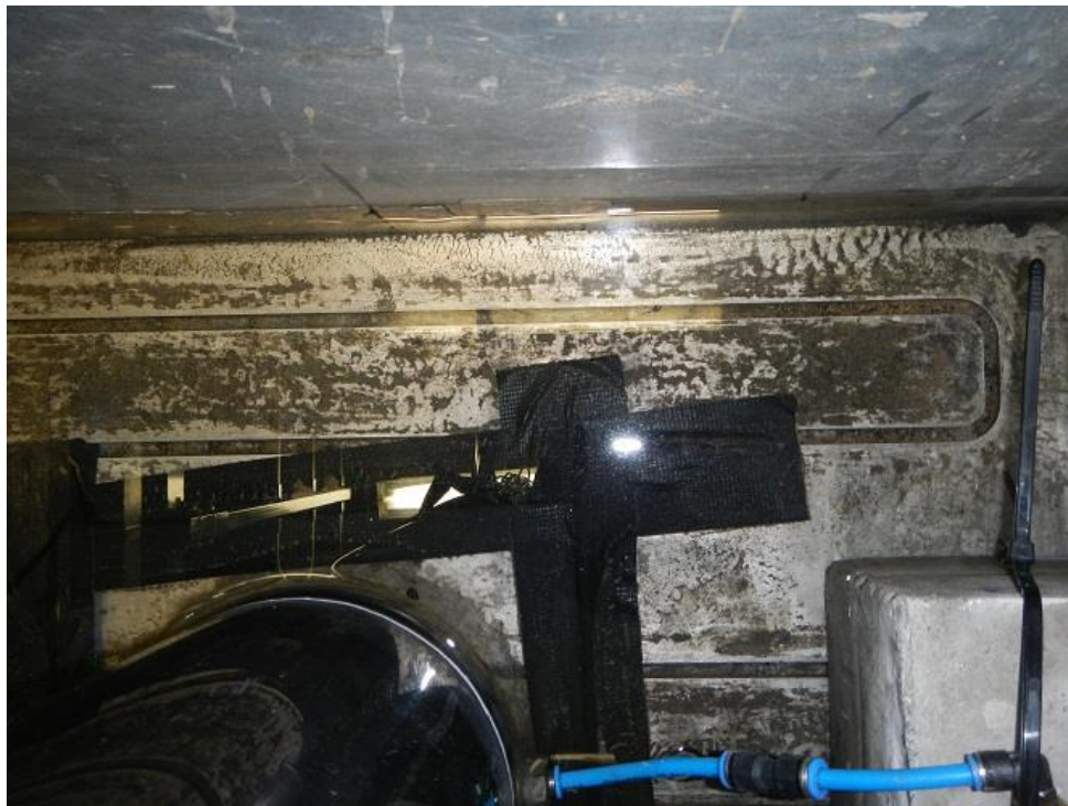
Figure 42: Particles observed on the bottom of the strongbox after completion of the full scale test.
