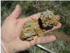
Figure A2: Redoximorphic features present at Q_Mid indicating signs of wetness
