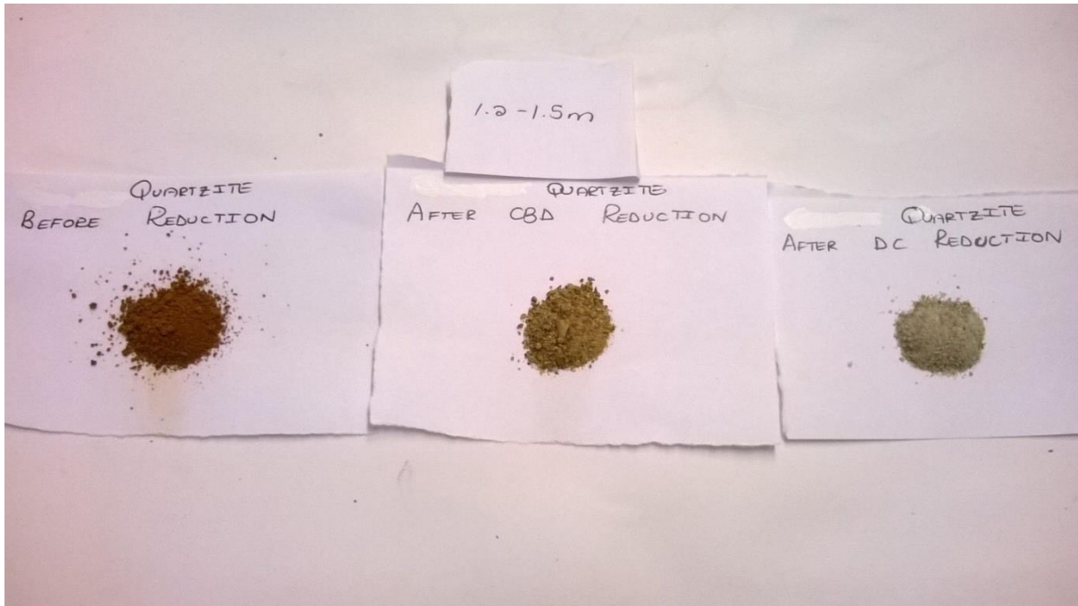
Figure 5.1: Q1_Crest_A showing extensive bleaching after CBD and complete bleaching after DC reduction
