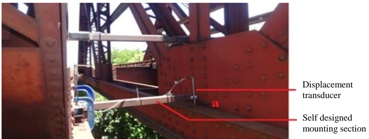
Figure 3.20: Displacement transducer fixed at point 'a'
