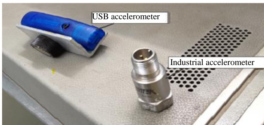
Figure 3.16: Closer view of USB and industrial accelerometer
