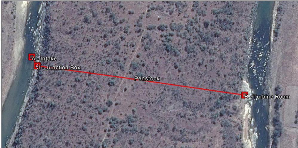
Figure 5-40 - Junction Box and Penstock - Mahlaba SSHP
