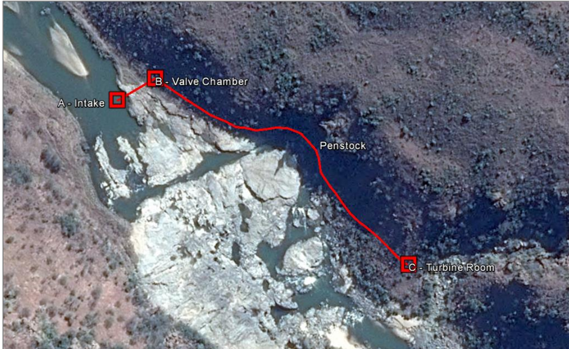
Figure 5-11 - Intake and penstock location and layout
