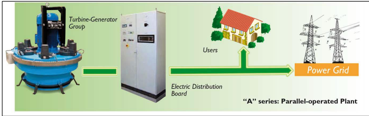
Figure 2-53 - Grid connected plant (Courtesy of IREM)
