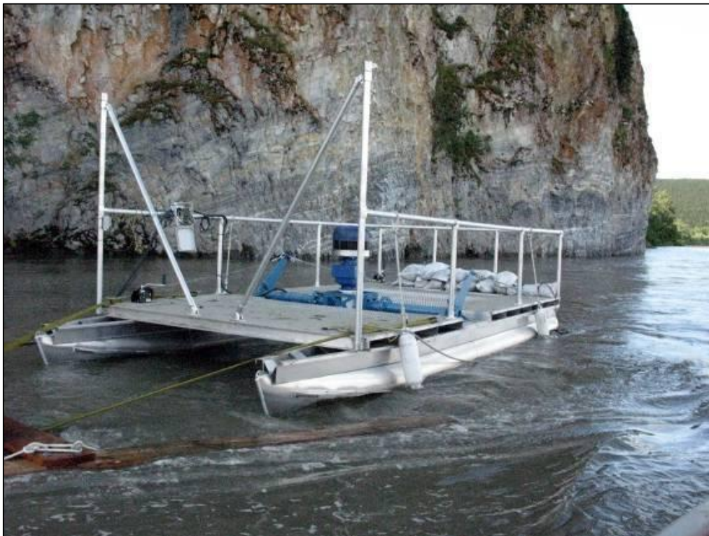
Figure 2-71 - Pontoon Boat with Encurrent Power Generation System (New Energy Corporation, 2015)
