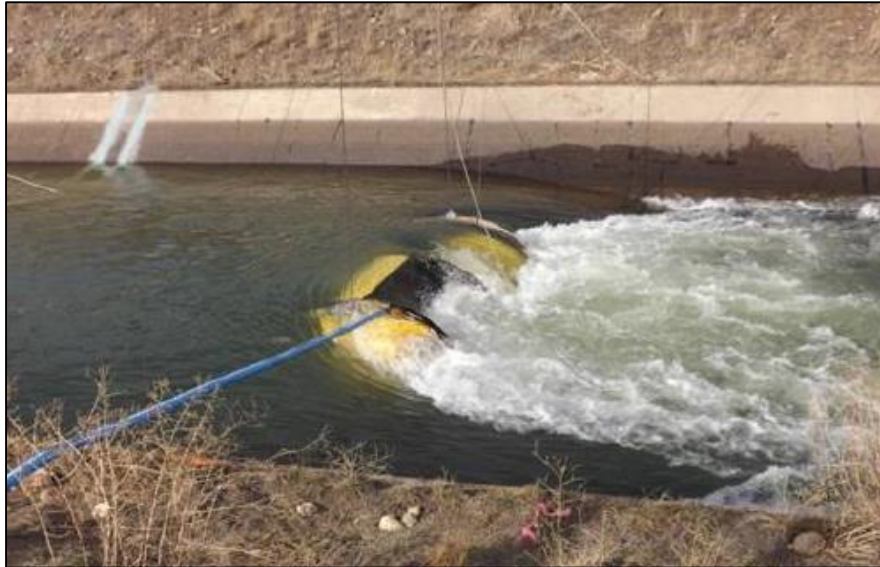
Figure 2-5 - Hydrovolts turbine installed in the Roza Canal in Oregon (Colorado Energy Office, 2007)
