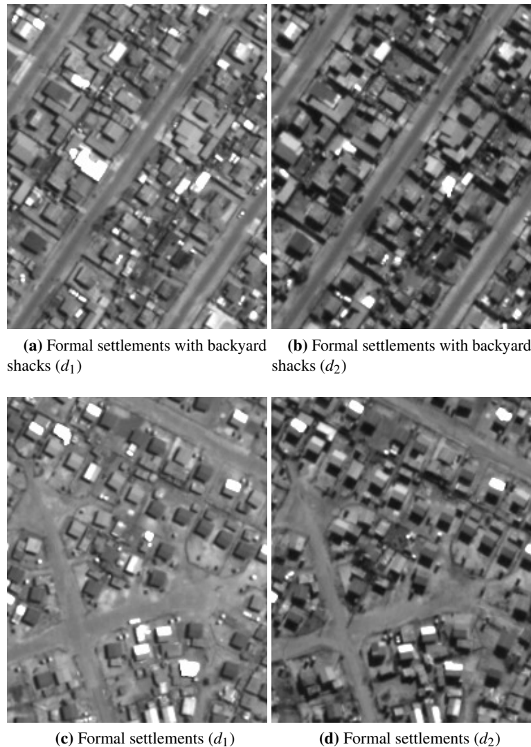
Figure 2.2. Shadow difference examples in urban land-use images for two different dates d_1 (early summer) and d_2 (early winter). Panchromatic QuickBird images courtesy of DigitalGlobe™.
