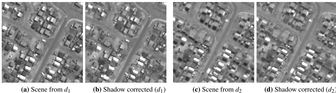
Figure 4.6. Illustration of the differences in shadow profiles for the same area acquired on different dates, and the corresponding scenes with fine shadow correction. (a) and (c) courtesy of DigitalGlobe™.
