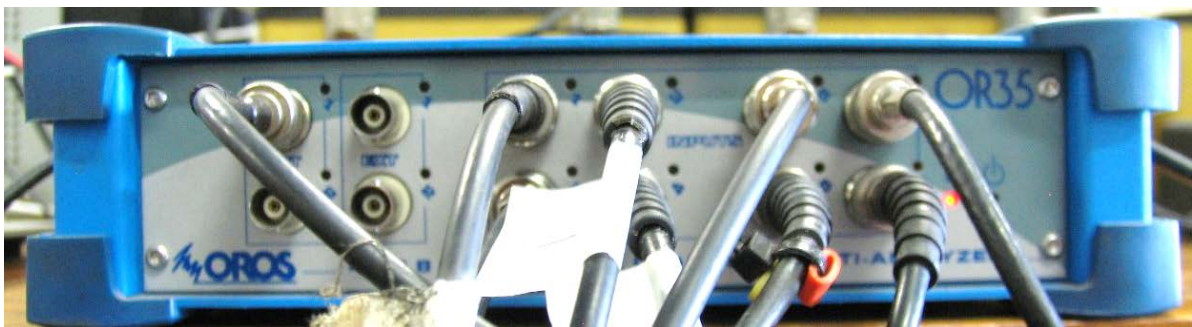
Figure 7.5-11 OROS OR35 data acquisition system
