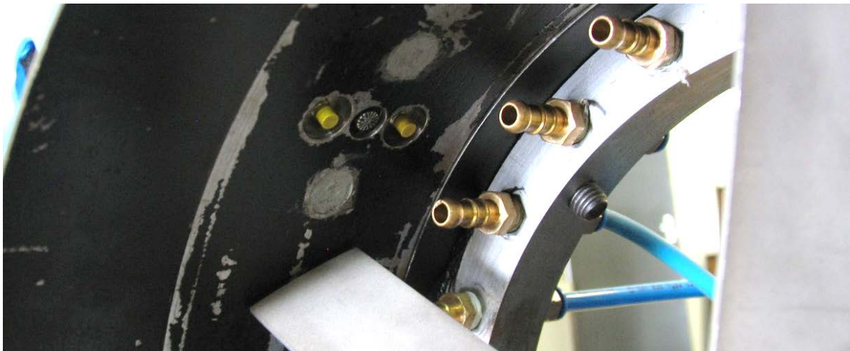
Figure 7.5-10 Inside view of drum with sensor plate, microphone and proximity transducers
