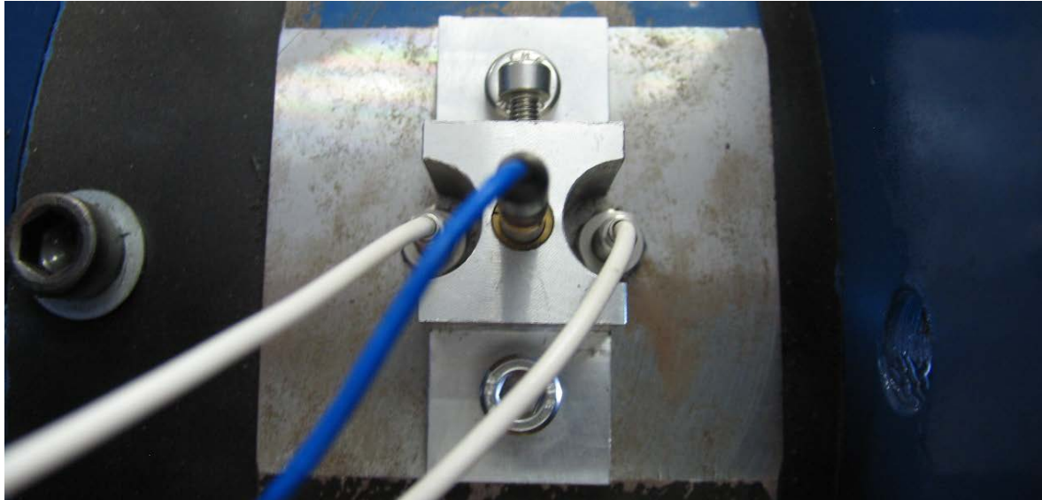
Figure 7.5-9 Sensor plate with attached microphone mount, microphone and proximity probes
