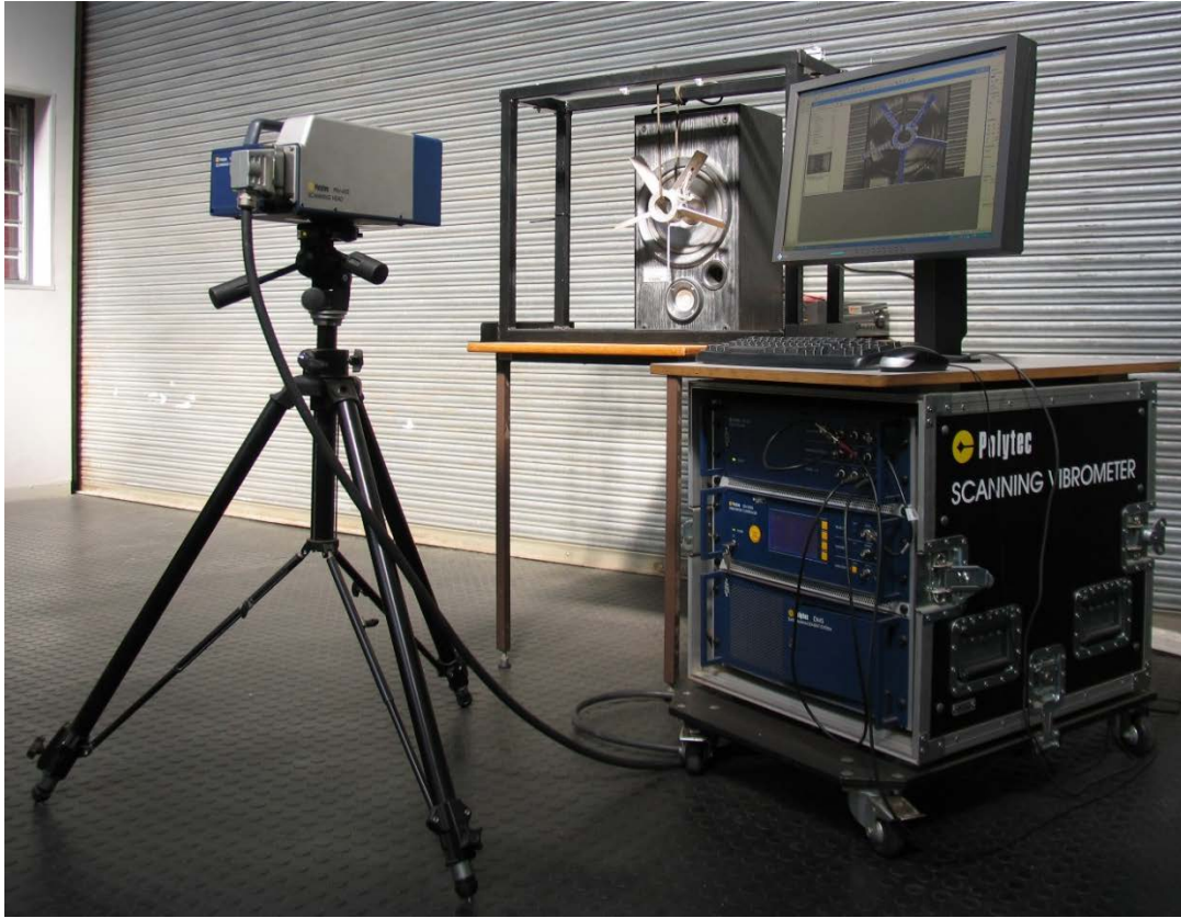
Figure 7.5-16 Scanning laser vibrometer set-up
