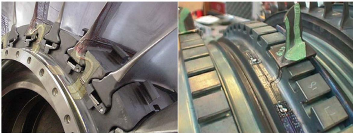
Figure 1.3-4 Example of rotor mounted strain gauges. (a) Root mounted strain gauges. (b) Blade mounted strain gauges. (Russhard, 2015)
