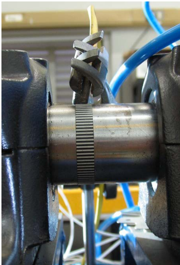
Figure 7.5-13 Shaft tachometer with 79 PPR zebra tape
